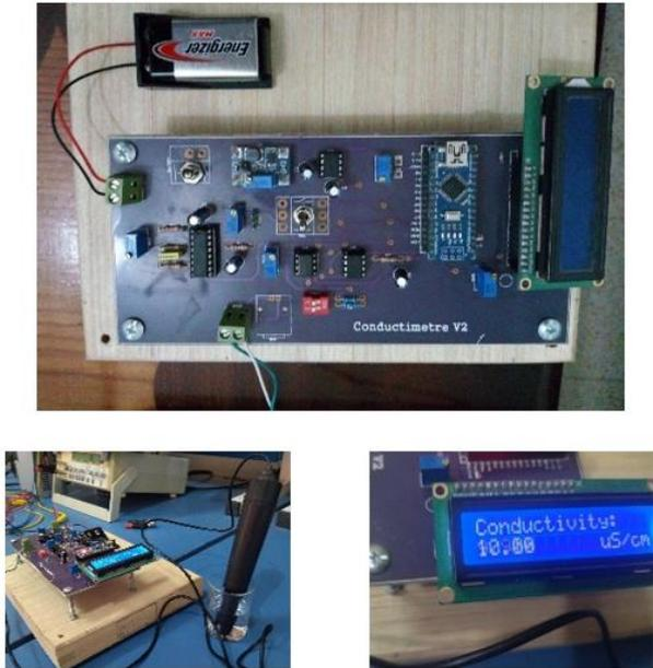
**Figure 6.** Photos of the designed device for measuring electrical conductivity
