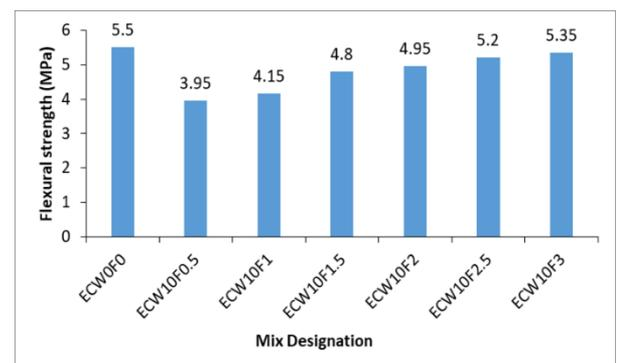
**Figure 8.** Flexural strength results of ECW and waste fibers-based mortars at 360 days
