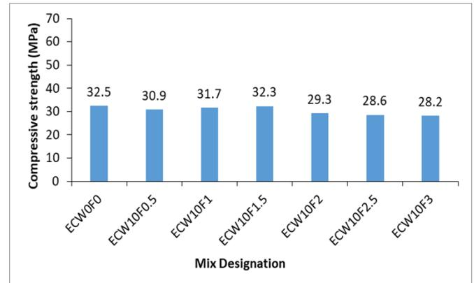
**Figure 3.** Compressive strength results of ECW and waste fibers-based mortars at 7 days
