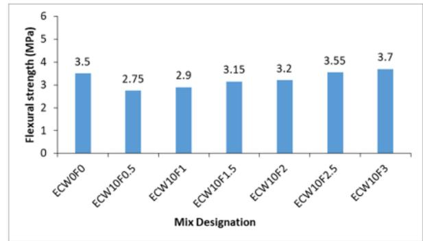
**Figure 6.** Flexural strength results of ECW and waste fibers-based mortars at 7 days
