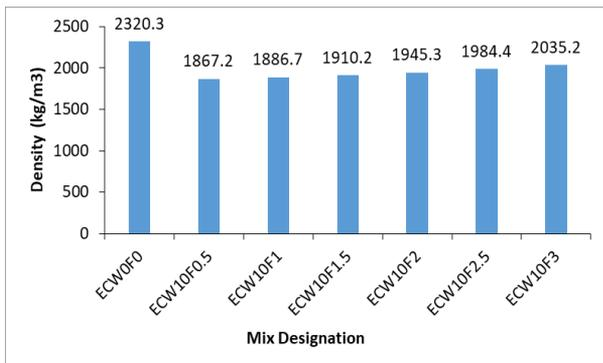
**Figure 10.** Bulk density results of ECW and waste fibers-based mortars at 28 days
