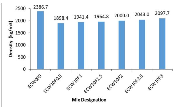
**Figure 11.** Bulk density results of ECW and waste fibers-based mortars at 360 days
