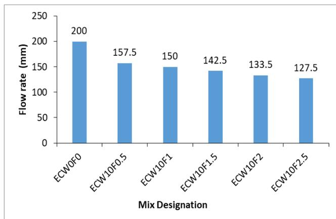
**Figure 2.** Flow rate results of ECW and waste fibers-based mortars
