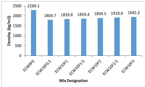
**Figure 9.** Bulk density outcomes of ECW and waste fibers-based mortar mixtures at 7 days
