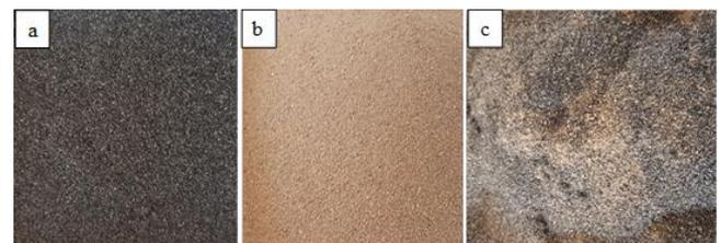
**Figure 1.** (a) Natural sand, (b) Electrical Cable Waste (ECW) aggregate and (c) mixing of the two types
