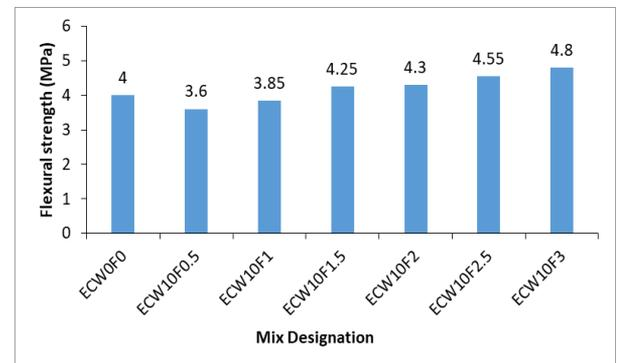
**Figure 7.** Flexural strength results of ECW and waste fibers-based mortars at 28 days
