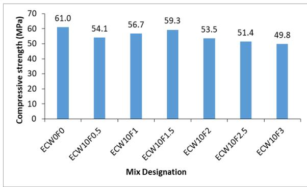
**Figure 5.** Compressive strength results of ECW and waste fibers-based mortars at 360 days
