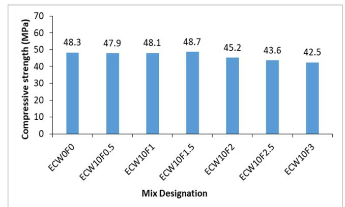
**Figure 4.** Compressive strength results of ECW and waste fibers-based mortars at 28 days
