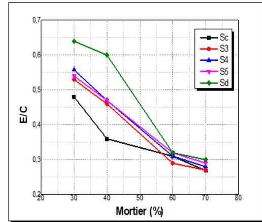
Figure 10. W/C ratio according to the % of mortar
