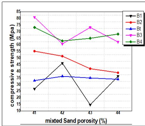
**Figure 13.** Effect of mixed sand porosity on the compressive strength at 28 days of the concrete
