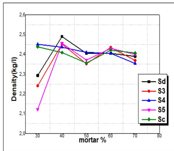
Figure 6. Density of the concretes according to the % of mortar
