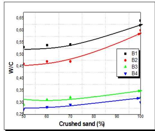
Figure 9. W/C ratio according to the % of crushed sand
