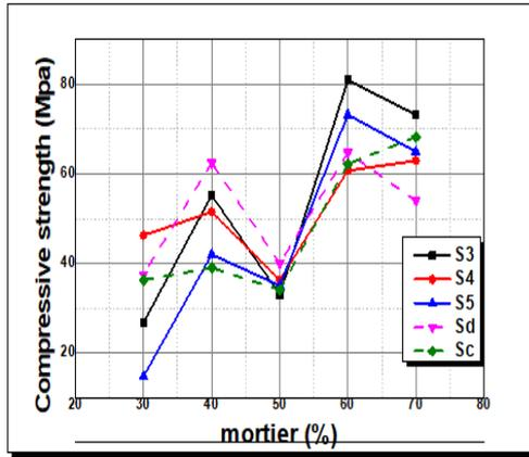
**Figure 12.** Variation of the compressive strength of concrete at 28 days according to the % of mortar
