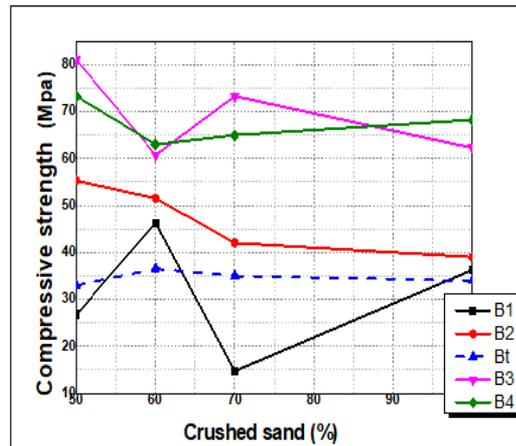
Figure 11. Variation of the compressive strength at 28 days according to the % of crushed sand
