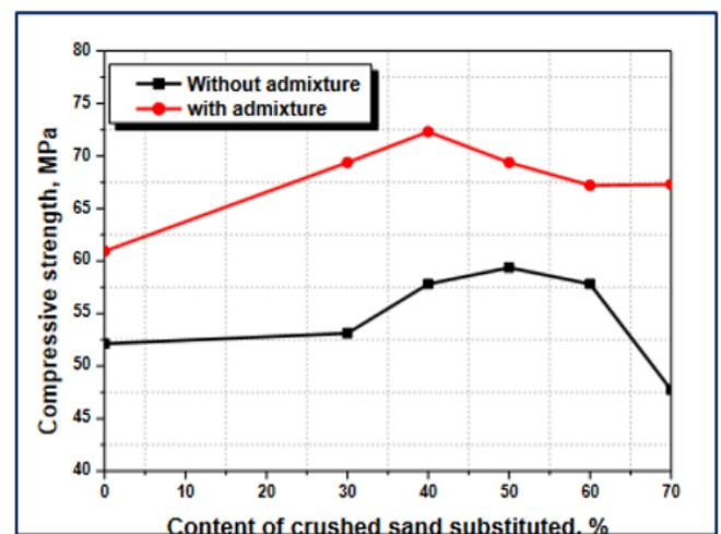
Figure 4. Compressive strength of mortars at 28 days according to the % of SC replaced [4]
