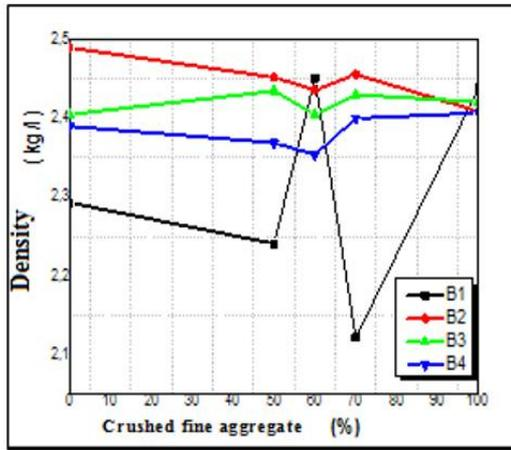
Figure 7. Density of the concretes according to the % of crushed sand
