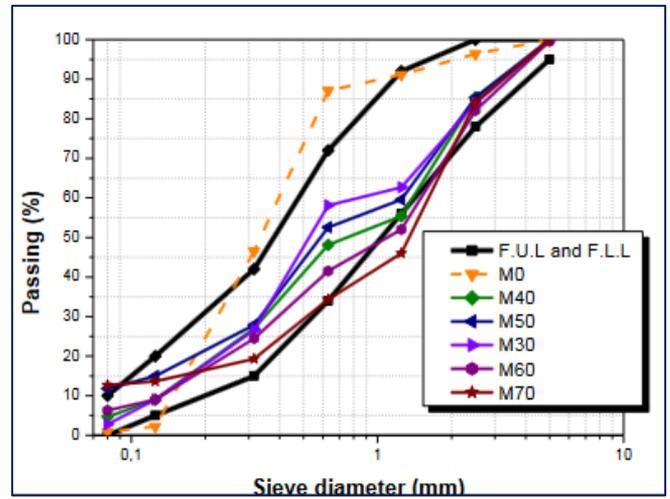
Figure 2. Grain size distribution of the mixed sand [4]
