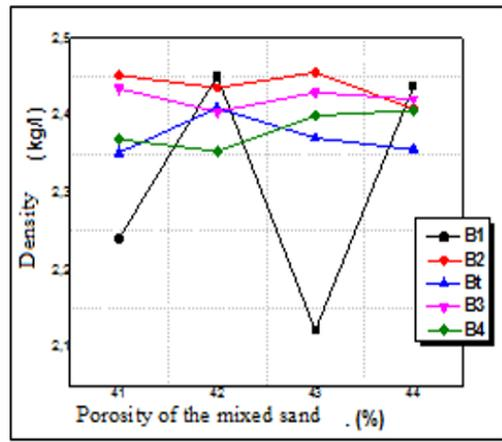
Figure 8. Density of the concretes according to the porosity of the mixed sand
