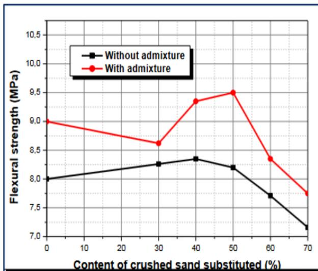
Figure 5. Variation of tensile strength of mortars at 28 days as a function of the quantity of SC substituted [4]
