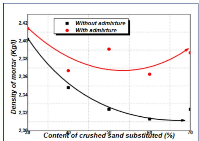
Figure 3. Density of mortars according to % of CS [4]
