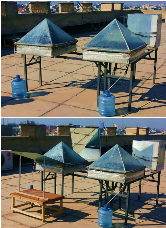
Figure 1. Experimental test-rig: (a) Solar stills without mirrors; (b) Solar stills with mirrors
