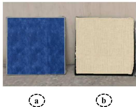
Figure 3. Photograph of various wick materials: (a) Velvet fabric; (b) Light cotton
