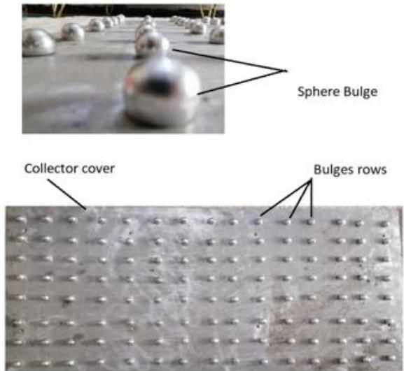
Figure 2. Structural pictures of an open-flow flat collector
