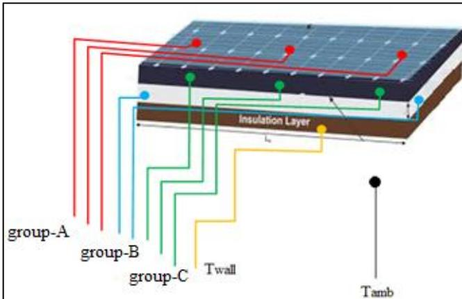
**Figure 3.** Positioning schematic of temperature measurement in the PV/T system
