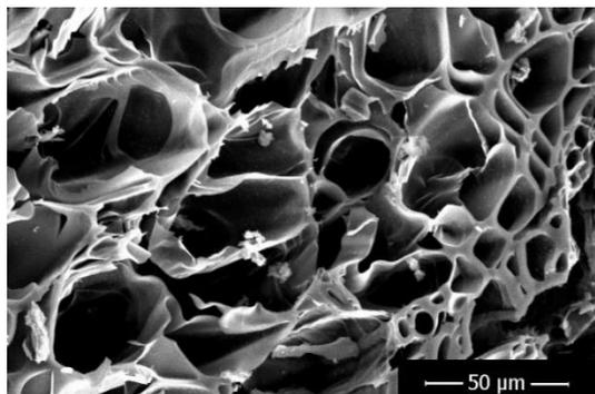
**Figure 9.** Biochar microstructure,  $2000\times$  magnification
