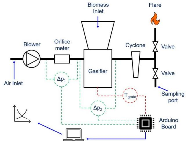
Figure 4. Scheme of the instrumented gasifier
