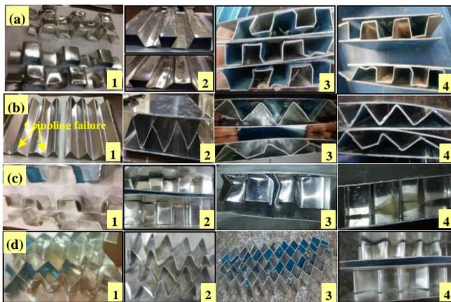
**Figure 5.** Compression failure modes for four sandwich structures (a) FS, (b) FT, (c) ES, and (d) ET cores at different stages under load
