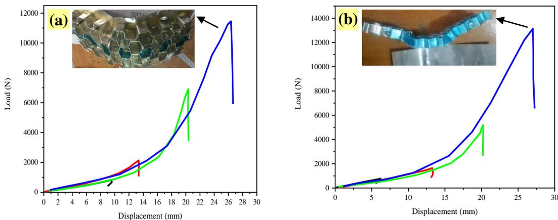
**Figure 7.** The load-displacement curves for sandwich panels with: (a) ES, and (b) ET cores under bending at different deflections (deflected panels, insets)
