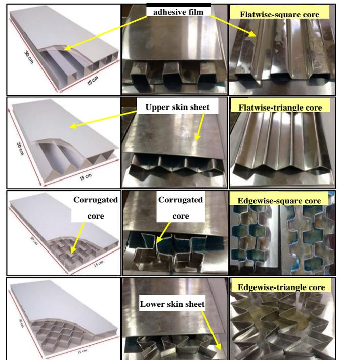
**Figure 2.** The four corrugated aluminum core arrangements: Flatwise Square (FS), Flatwise Triangle (FT), Edgewise Square (ES), and Edgewise Triangle (ET)
