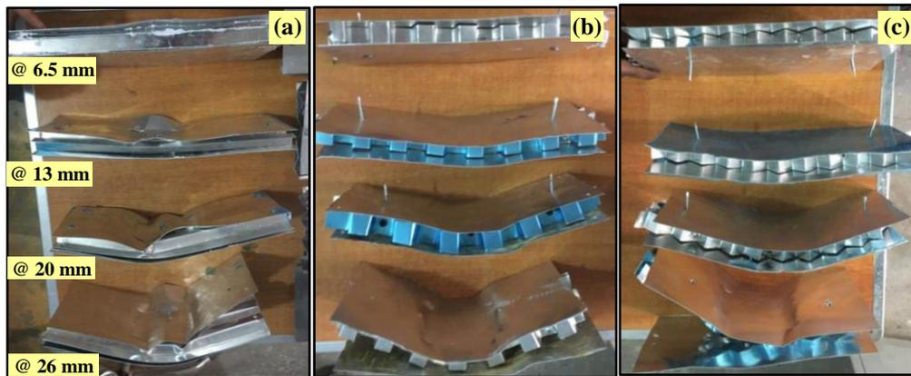
**Figure 8.** Deformed panels after bending at different deflections (6.5, 13, 20, 26 mm) with: (a) FS, (b) ES, and (c) ET
