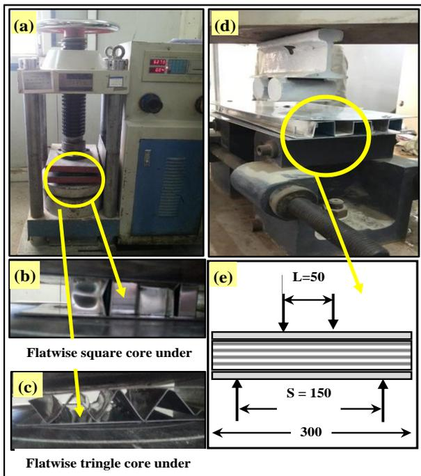
**Figure 3.** (a) the compression machine; (b & c) the FS and FT cores under compression; (d) the universal testing machine; and (e) four-point bending configuration
