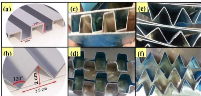
**Figure 1.** The corrugated square and tringle cores (a & b); flatwise square (FS) and edgewise square (ES) (c & d); and flatwise triangle (FT) and edgewise triangle (ET) (e & f)
