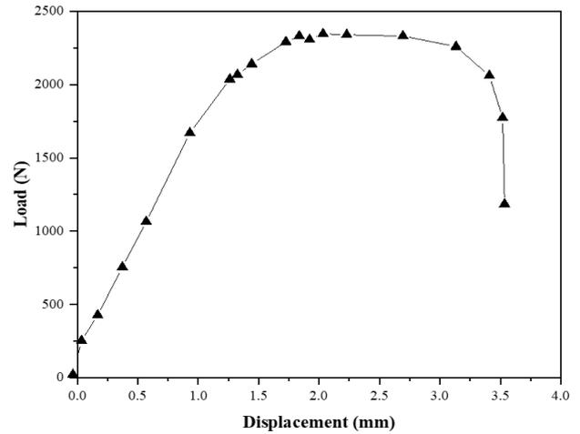
**Figure 4.** The load-displacement curve for aluminum facesheets
