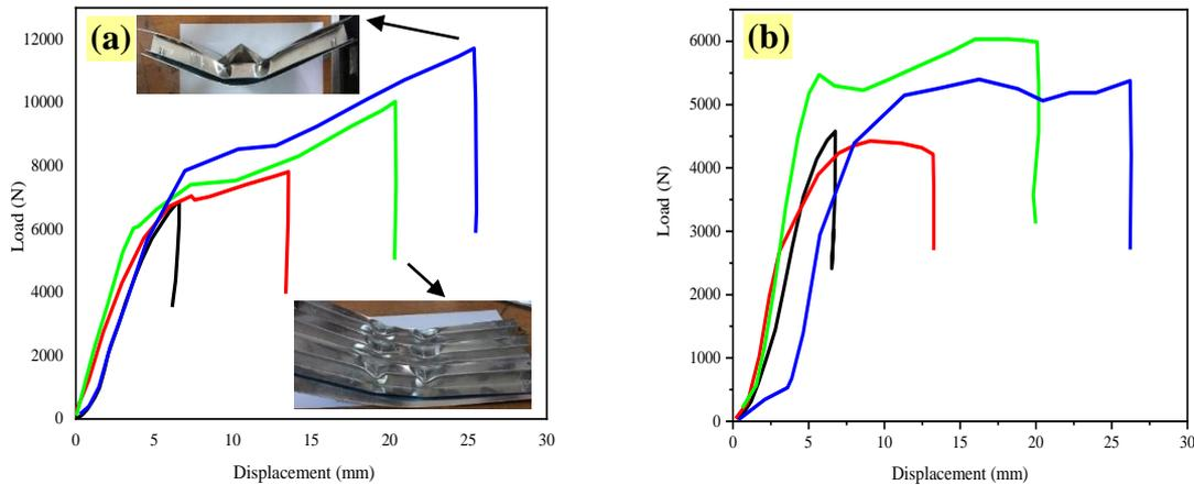
**Figure 6.** The load-displacement curves for sandwich panels with: (a) FS (deflected panels, insets), and (b) FT cores under bending at different deflections
