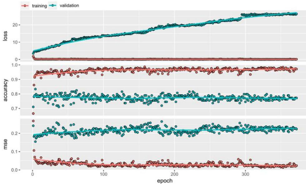
Figure 2. Training process of the two-neuron classifier without hidden layers
