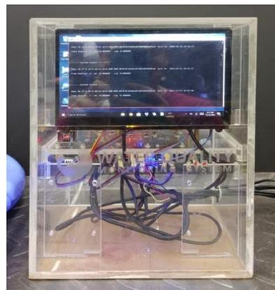
**Figure 4.** Front view of node station hardware implementation
