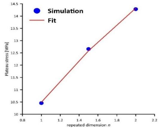
**Figure 19.** Comparison between plateau stress of fitted and numerical results
