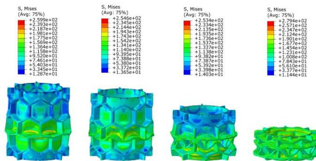
Figure 9. Captured deformation pattern in the internal geometry of the original structure L
