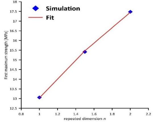
**Figure 18.** Comparison between collapse stress of fitted and numerical results
