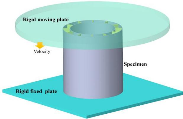
Figure 6. Illustration of the compression test configuration
