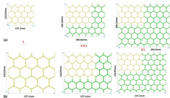
Figure 3. New structures containing more cells, and the same dimension and density as in the original structure (a): before the scale and (b) after the scale
