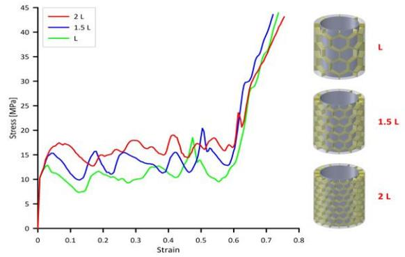
**Figure 14.** Resulting stress-strain compressive curves for the three tested honeycomb-filled double circular tubes
