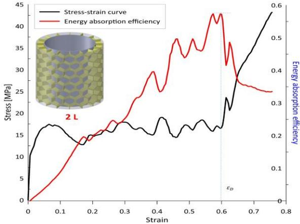
**Figure 17.** Efficiency-strain and stress-strain curves of total-duplicated structure 2L
