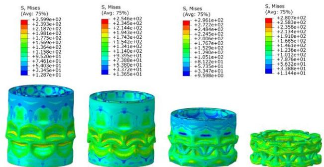
Figure 8. Deformation pattern and von mises stress distribution in the original structure L during the compression test
