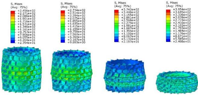
**Figure 13.** Captured deformation pattern in the internal geometry of the total-duplicated structure 2L
