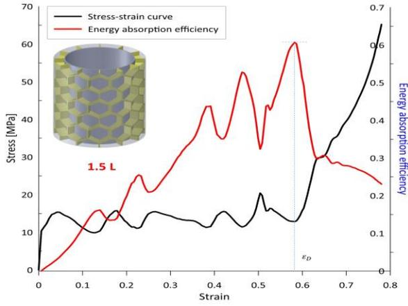
**Figure 16.** Efficiency-strain and stress-strain curves of half-duplicated structure 1.5 L
