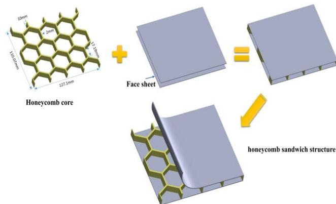
Figure 1. Designed honeycomb sandwich panel structure
