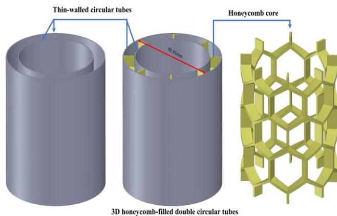
Figure 2. Schematic illustration of the created cylindrical honeycomb sandwich structure
