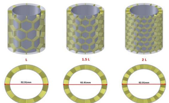
Figure 5. Cylindrical honeycomb sandwich structures designed with an increased number of cells and constant dimensions
