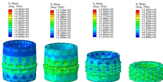
Figure 10. Deformation pattern and von mises stress distribution in the half-duplicated structure 1.5 L during the compression test
