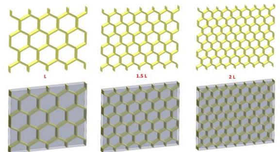
Figure 4. Schematic illustration of honeycomb sandwich structures designed with an increased number of cells and constant dimensions
