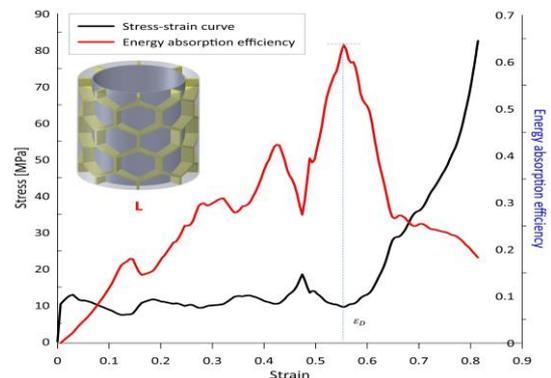
**Figure 15.** Efficiency-strain and stress-strain curves of original structure L
