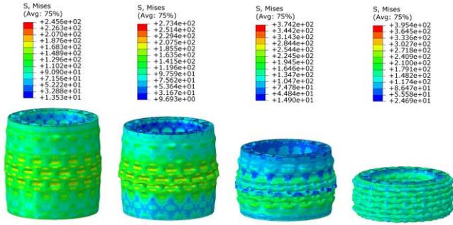
**Figure 12.** Deformation pattern and von misses stress distribution in the total-duplicated structure 2L during the compression test
