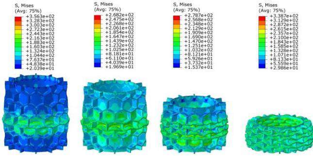
**Figure 11.** Captured deformation pattern in the internal geometry of the half-duplicated structure 1.5L
