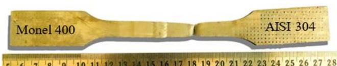
Figure 6. ASTM E8 standard tensile samples (fracture sample)
