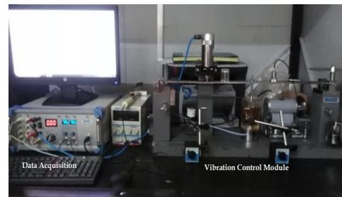
**Figure 2.** Vibration fundamental trainer
