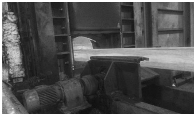
Figure 3. Hot charge entering the furnace
