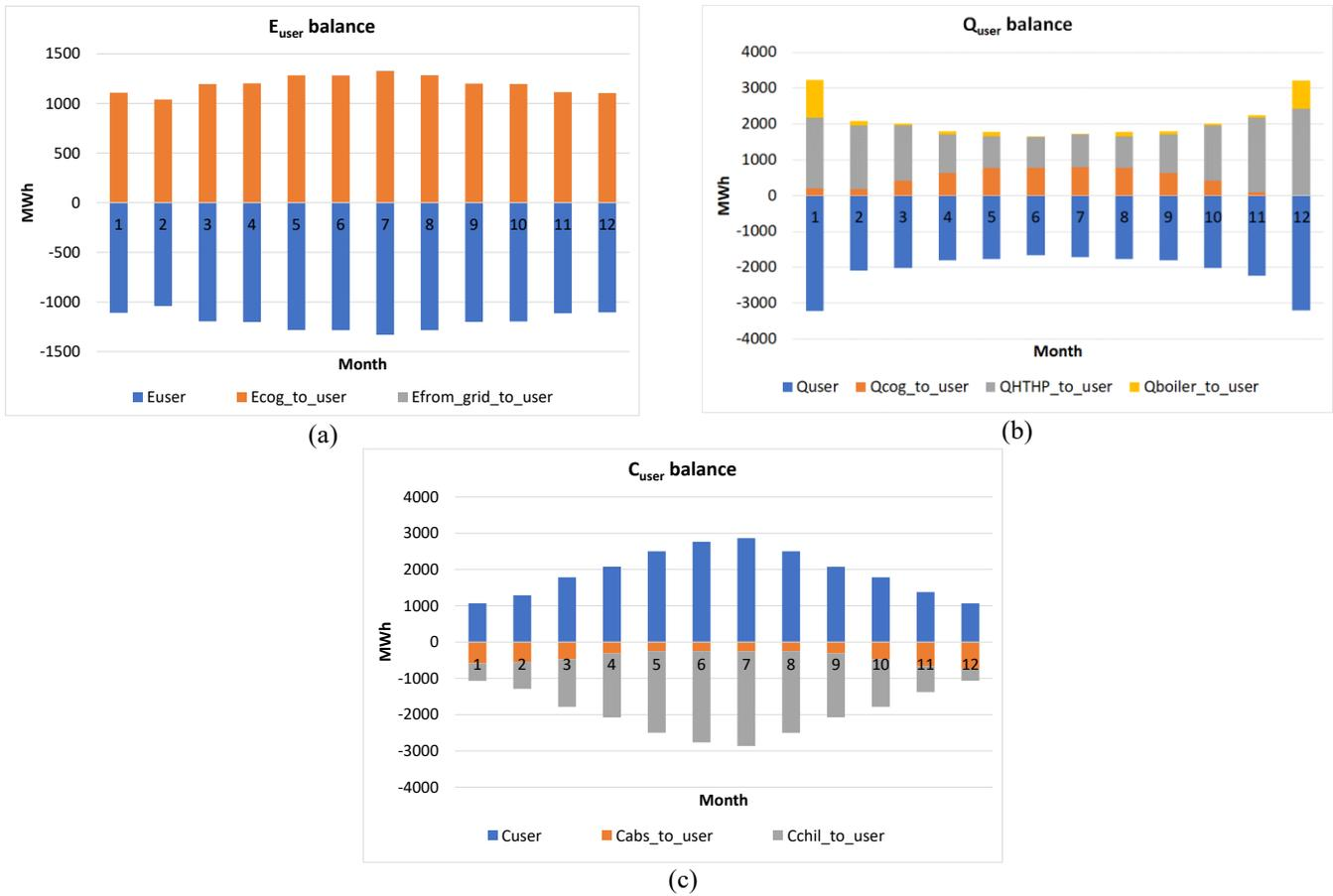
**Figure 6.** Monthly energy balance of the user's electricity demand (a), thermal energy demand (b) and cooling energy demand (c)
