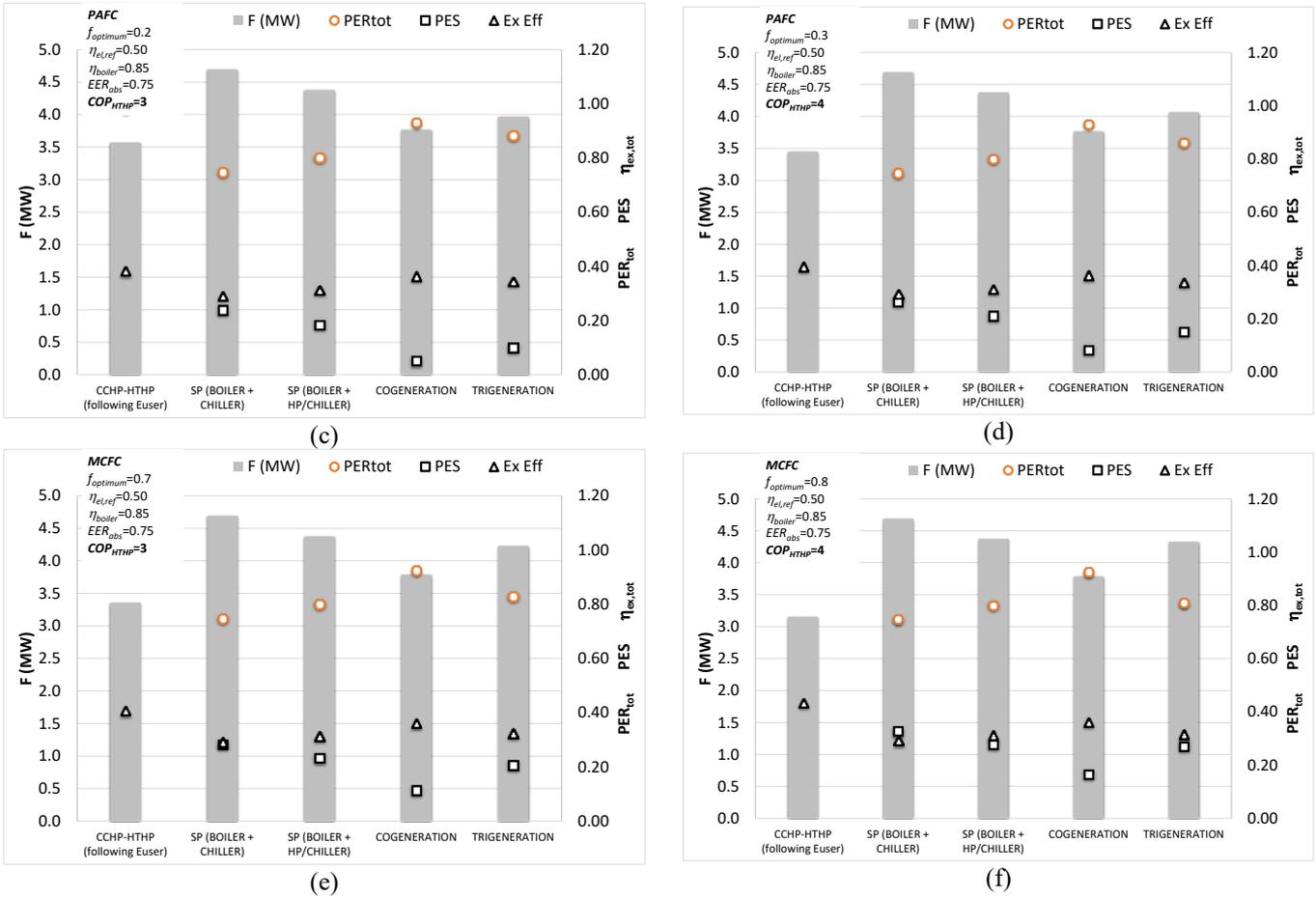
**Figure 4.** Non-primary energy power input ( $F$ ), energy and exergy performance ( $PER_{tot}$  and  $\eta_{ex,tot}$ , respectively) of the systems, and primary energy savings ( $PES$ ) of CCHP+HTHP with respect to the benchmark systems
