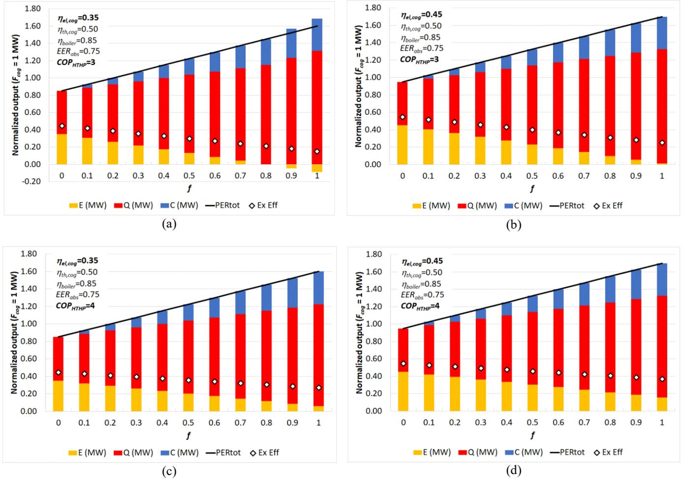
**Figure 2.** Power output, energy and exergy performance of the CCHP+HTHP system varying the fraction of cogeneration recovery heat to cooling ( $f$ ) for 1 MW of NG input ( $\eta_{el,ref}=0.5$ )
