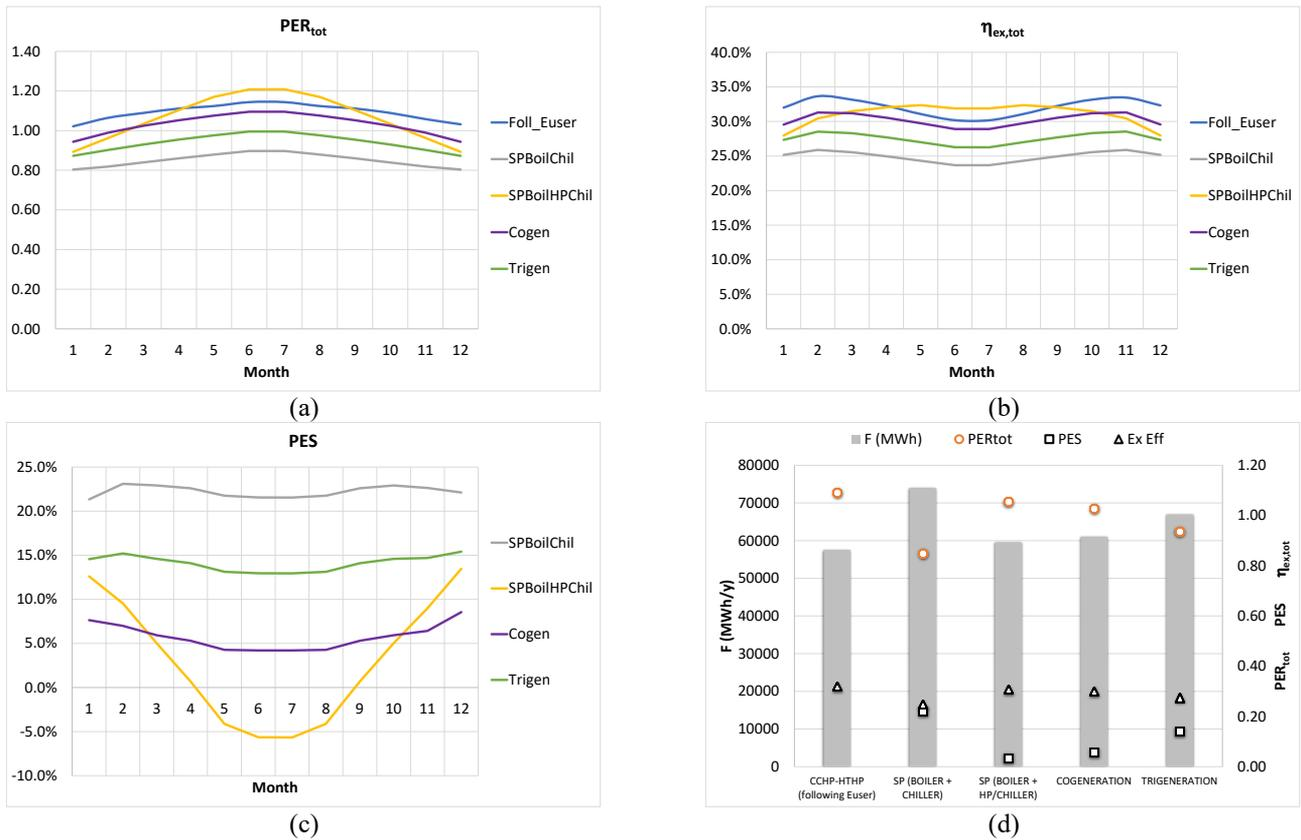
**Figure 5.** Monthly values of the primary energy ratio (a), exergy efficiency (b), and primary energy saving (c) of CCHP+HTHP with respect to the benchmark systems; annual values of energy performance of the systems (d) (with optimized values of  $f$  for each month)
