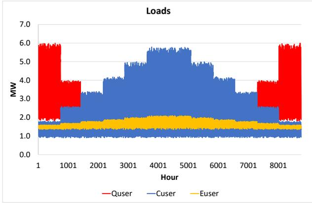
**Figure 3.** Electric ( $E_{user}$ ), thermal ( $Q_{user}$ ) and cooling ( $C_{user}$ ) hourly loads for the annual simulation
