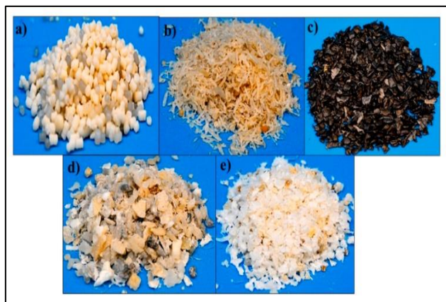
Figure 4. RPA categories used to substitute natural coarse aggregates: (a) Granules, (b) Fibers, (c) Black flakes, (d) Mixed flakes and (e) White flakes [5]
