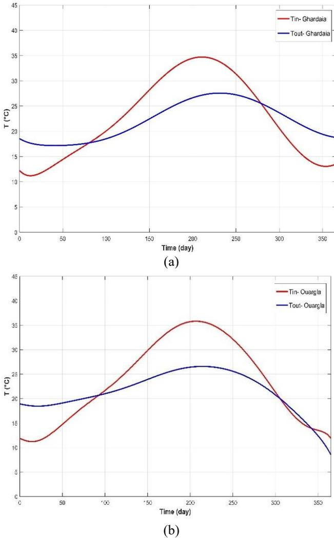
**Figure 5.** Evolution of inlet and outlet EAHE temperatures: (a) Ghardaia region, (b) Ouargla region
