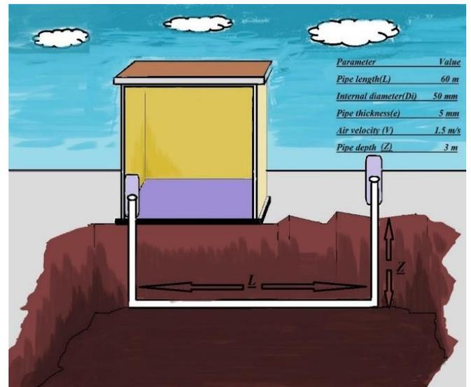
Figure 1. Diagram of EAHE system
