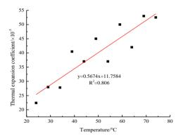
Figure 3. Thermal expansion coefficients of the bolting system at different temperatures
