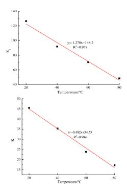
Figure 5. Relationship between tensile shear stiffness and temperature
