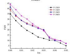
Figure 7. Axial force distributions of the bolts at different loads
