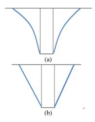
Figure 1. The shape of the failure surface of the shearing cone
