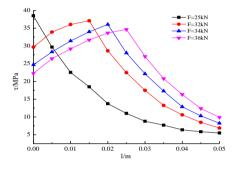
Figure 6. Shear stress distributions of the bolts at different loads
