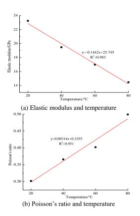
Figure 2. Deformation parameters of the bolting system at different temperatures
