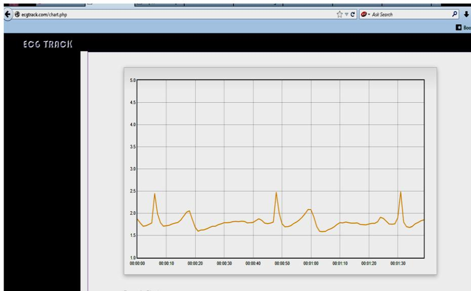
**Figure 8.** Screen shot of the potted ECG waveform in the web browser
