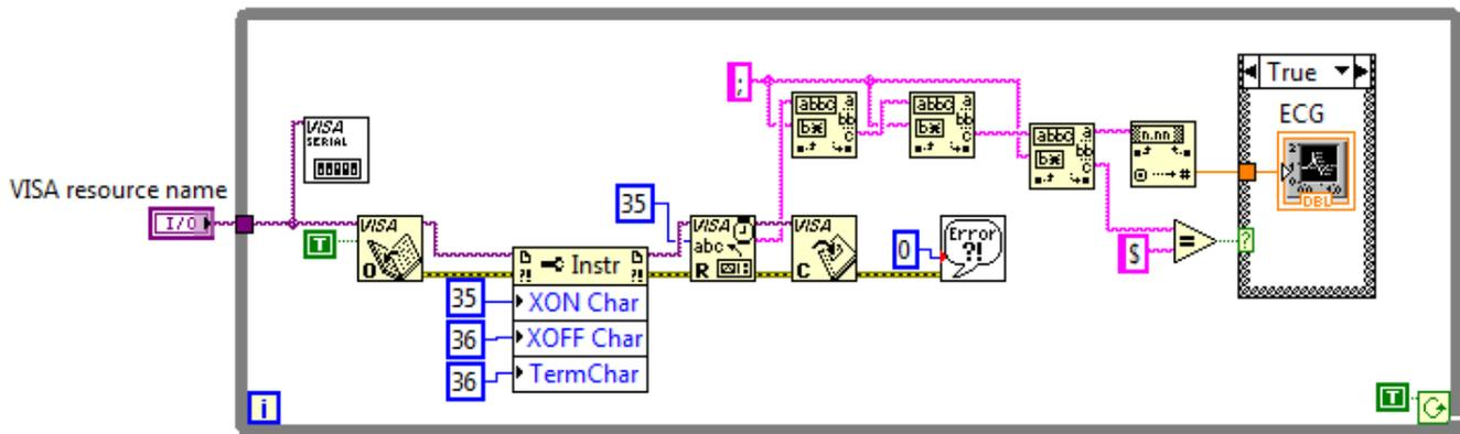
**Figure 3.** Block diagram for ECG display in Lab VIEW
