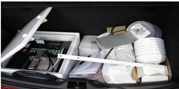
**Figure 3.** Babuc ABC data logger: central unit and probes
