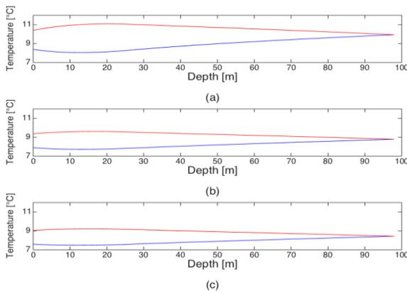
**Figure 7.** Temperature profiles in the downward (blue) and upward (red) pipe for exchanger B1 in I2
