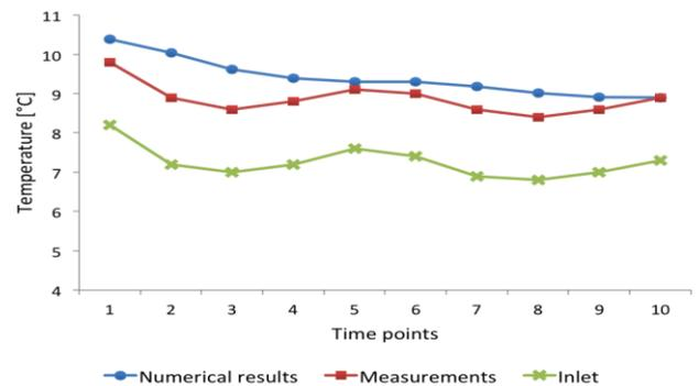
**Figure 4.** Comparison between numerical and real temperatures on the outlet face of exchanger B2 in the time interval I1
