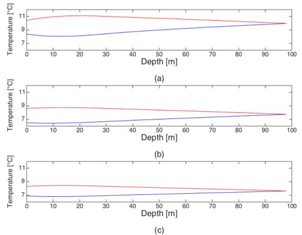
**Figure 8.** Temperature profiles in the downward (blue) and upward (red) pipe for exchanger B1 in I2
