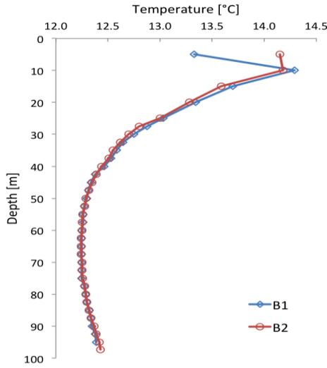
**Figure 2.** Undisturbed temperature profiles measured in boreholes B1 and B2
