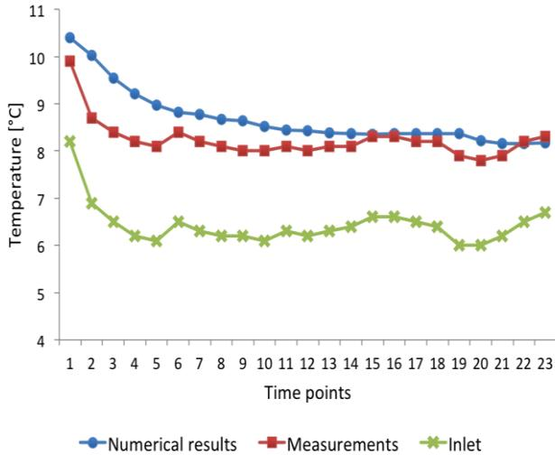
**Figure 6.** Comparison between numerical and real temperatures on the outlet face of exchanger B2 in the time interval I2
