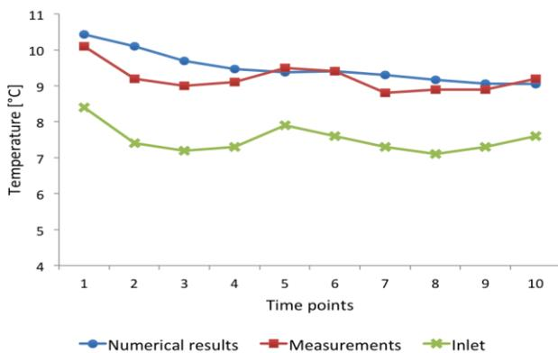
**Figure 3.** Comparison between numerical and real temperatures on the outlet face of exchanger B1 in the time interval I1
