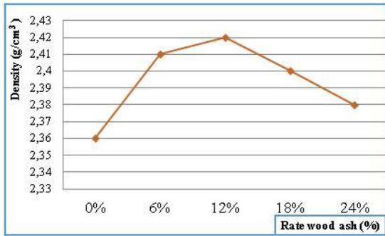
Figure 7. Effect of the substitution rate on the density
