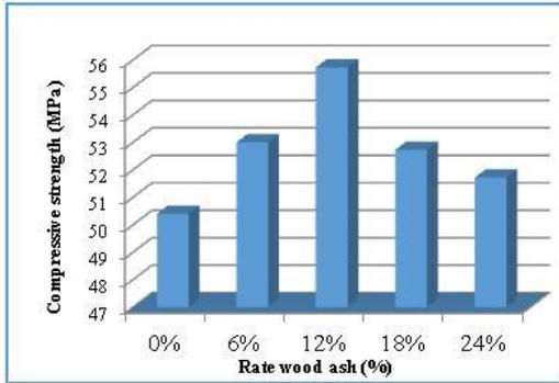
Figure 12. Compressive strength obtained by rebound hammer testing
