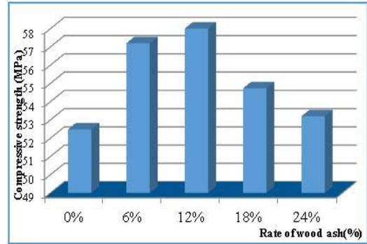
Figure 14. Influence of the substitution rate on the compressive strength obtained by combined method
