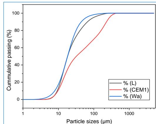
**Figure 1.** Particle size distribution of cement, limestone and wood ash
