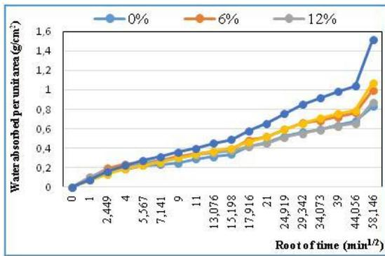
Figure 17. Variation of absorption by capillarity as a function of root of time
