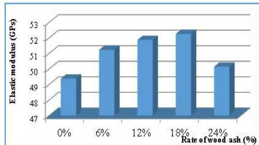
Figure 15. Relationship of elastic modulus with wood ash content
