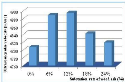
Figure 13. Variation of ultrasonic pulse velocity as a function of substitution rate of wood ash
