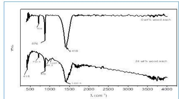
Figure 20. FTIR of SCCs of 0 and 24% wood ash
