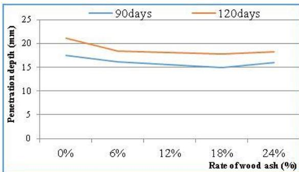
Figure 18. Variation in depth of chloride penetration containing wood ash
