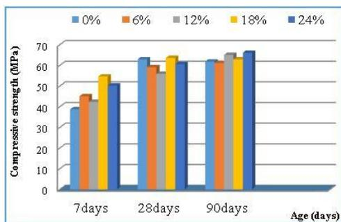
Figure 9. Effect of the substitution rate of wood ash on the compressive strength
