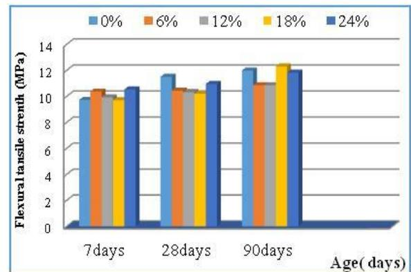
Figure 11. Effect of the substitution rate of wood ash on the flexural tensile strength
