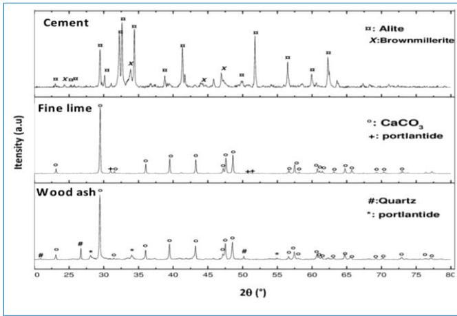
**Figure 2.** XRD patterns of Portland cement, fine limestone and wood ash
