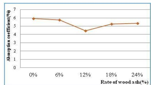
Figure 16. Effect of substitution rate on water absorption variation
