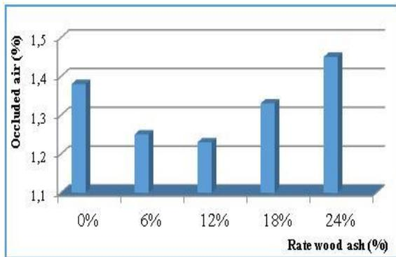
Figure 8. Effect of the substitution rate on the occluded air variation
