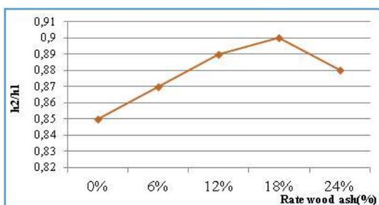
Figure 4. The impact of substitution rate on the passing ability
