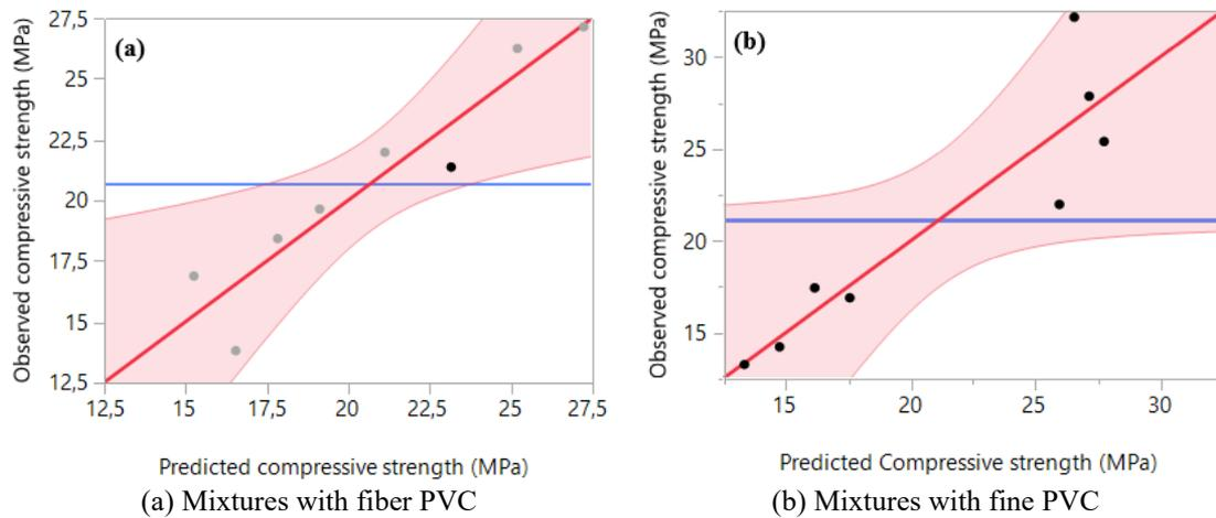
**Figure 9.** Correlation between the observed and the predicted compressive strength
