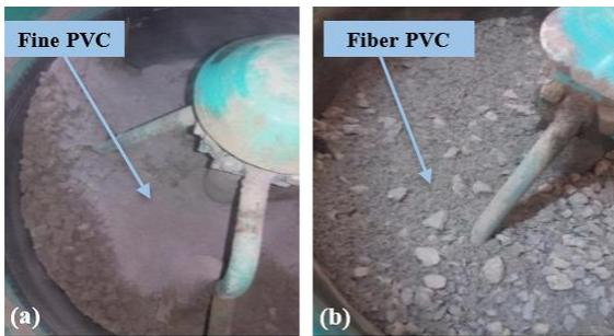
**Figure 3.** Concrete mixtures with different PVC waste: (a) Fine PVC aggregate and (b) Fiber PVC
