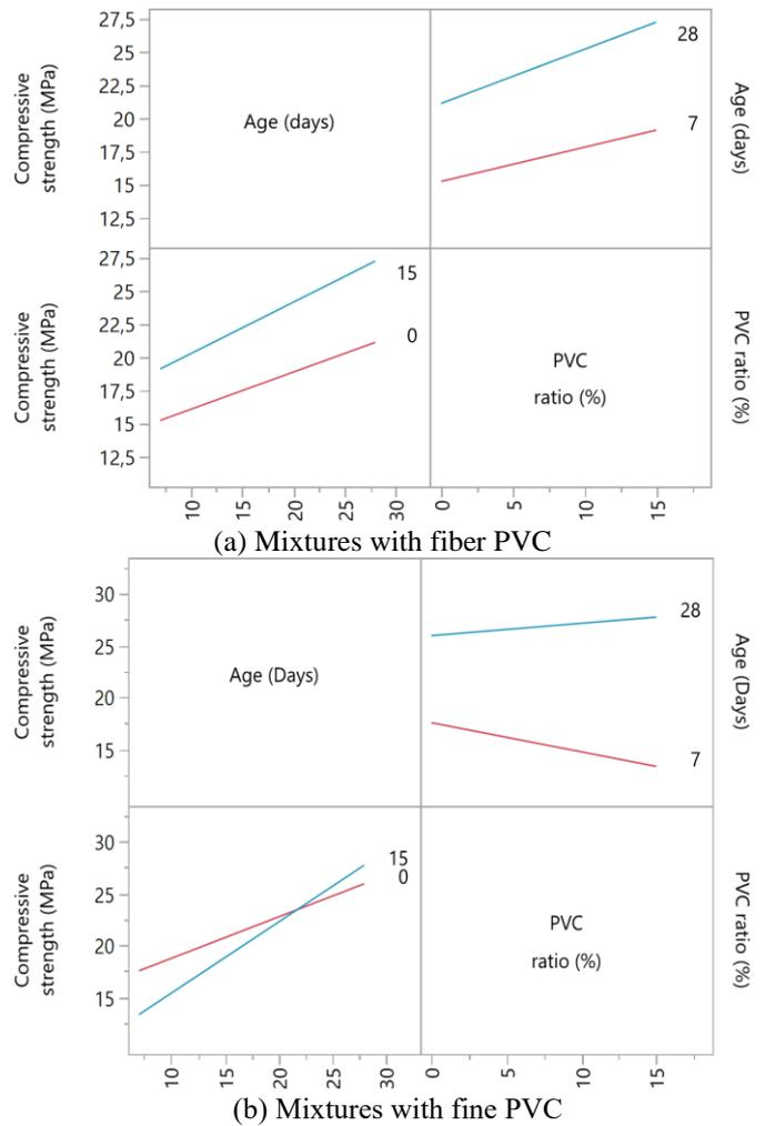
**Figure 11.** Interaction plot of compressive strengths for different concrete mixes
