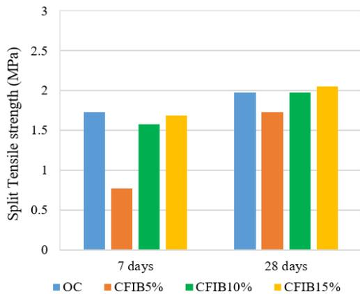
(a) Split tensile strength of concrete with PVC Fiber
