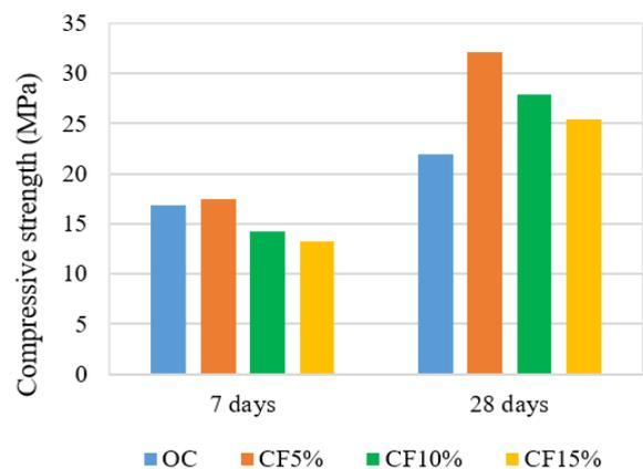
(b) Compressive strength of concrete with PVC Fine
