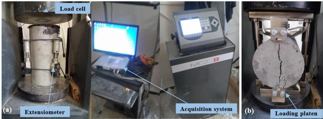
Figure 6. (a) Compressive strength test and (b) Split tensile strength test
