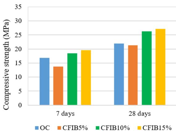
(a) Compressive strength of concrete with PVC Fiber
