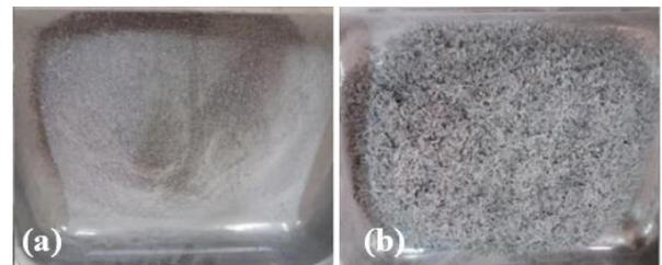
**Figure 2.** Crushed PVC waste: (a) Fine PVC and (b) Fiber PVC
