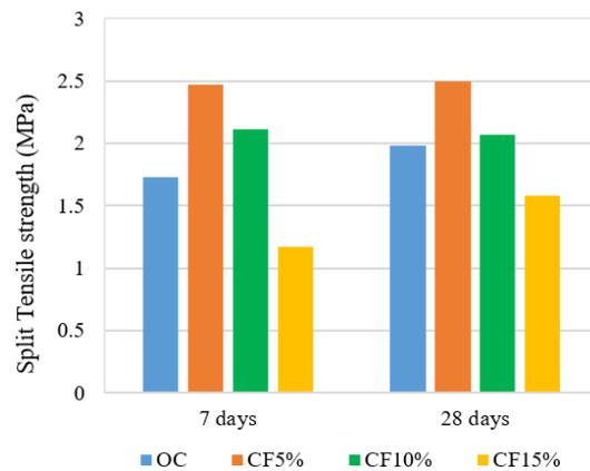
(b) Split tensile strength of concrete with PVC Fine
