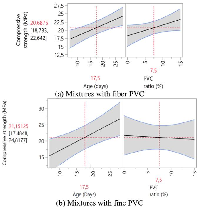
**Figure 10.** Main effect plot for different concrete mixes
