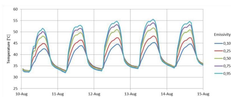
Figure 9: Temperature values inside the cabinet for several emissivity values.
