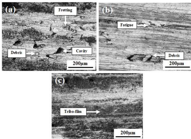
Figure 8. The AMC worn surfaces at 25N normal applied load; (a) S1, (b) S2, and (c) S3
