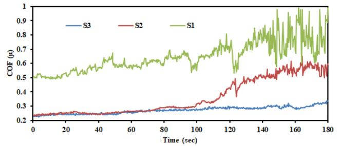
**Figure 4.** Coefficient of friction behaviors of AA6061/Gr/Al<sub>2</sub>O<sub>3</sub> composites
