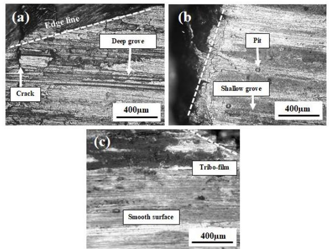
**Figure 5.** Frictional AMC surfaces at 20N normal applied load; (a) S1, (b) S2, (c) S3
