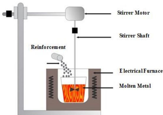
**Figure 1.** The stir casting technique
