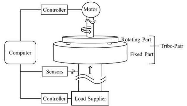
**Figure 2.** Schematic of the pin on disc tribometer
