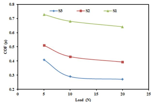
**Figure 6.** The effect of Al<sub>2</sub>O<sub>3</sub>/Gr content on the coefficient of friction of AMC under multi-applied loads
