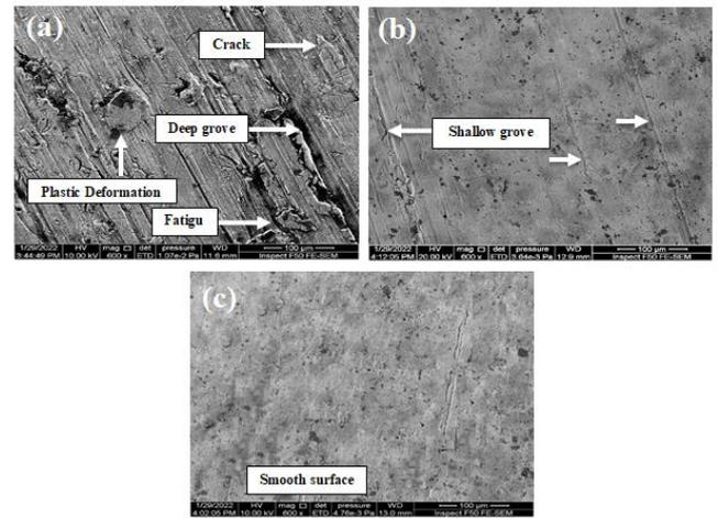
Figure 10. Scanning electronic microscope of AMC worn surfaces at 15N normal applied load and 1750m sliding distance; (a) S1, (b) S2, (c) S3
