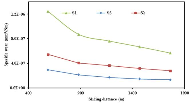
Figure 9. The relations of AMC specific wear with sliding distance
