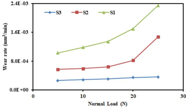
Figure 7. The effect of reinforcement and loads on the wear rate of AA6061
