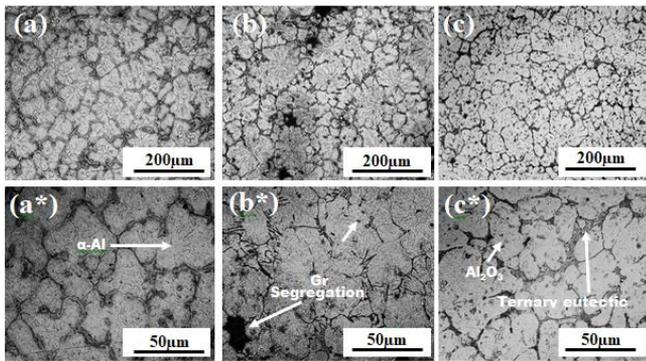
**Figure 3.** The optical microstructure of the AMC: (a,a\*) AA6061, (b,b\*) AA6061 with 5wt% Gr, (c,c\*) AA6061 with 5wt% Gr and 5 wt% Al<sub>2</sub>O<sub>3</sub>
