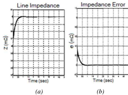
Figure 6. (a) Line impedance (b) Impedance Error of current control loop with sinusoidal current
