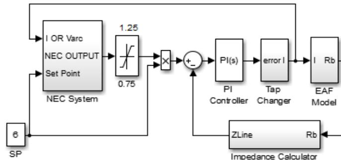
Figure 9. Controller loop with NEC implementation
