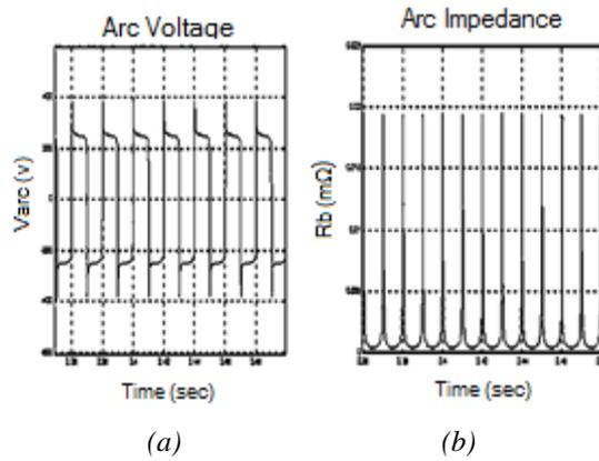
Figure 5. (a) Arc Voltage, (b) Arc Impedance of current control loop with sinusoidal current
