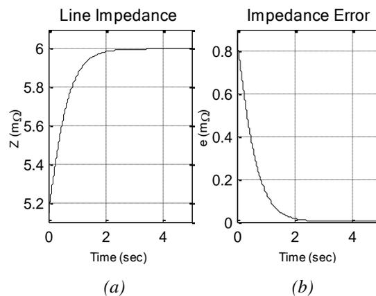
Figure 7. (a) Line Impedance (b) Impedance Error of current control loop with RMS current
