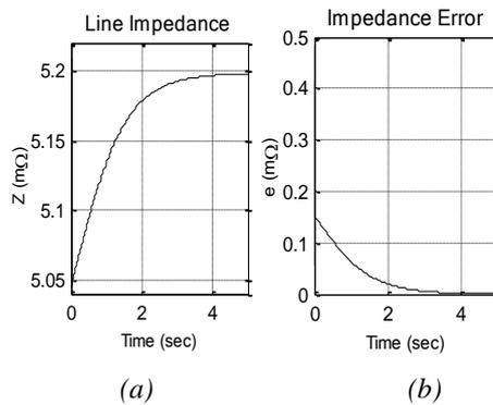
Figure 11. (a) Line Impedance (b) Impedance Error of control loop with NEC implementation
