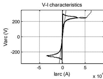
Figure 1. Voltage-current characteristics of arc
