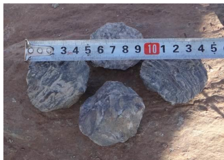
Figure 11. Large-grain rock blocks discharged from the reverse circulation
