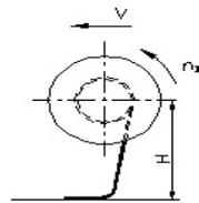
Figure 5. Schematic diagram of cable position when reel stops
