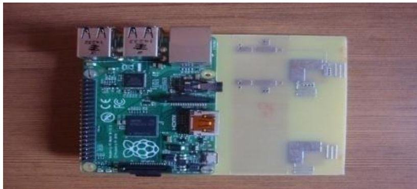
Figure 3. Reconfigurable antenna with Raspberry Pi
