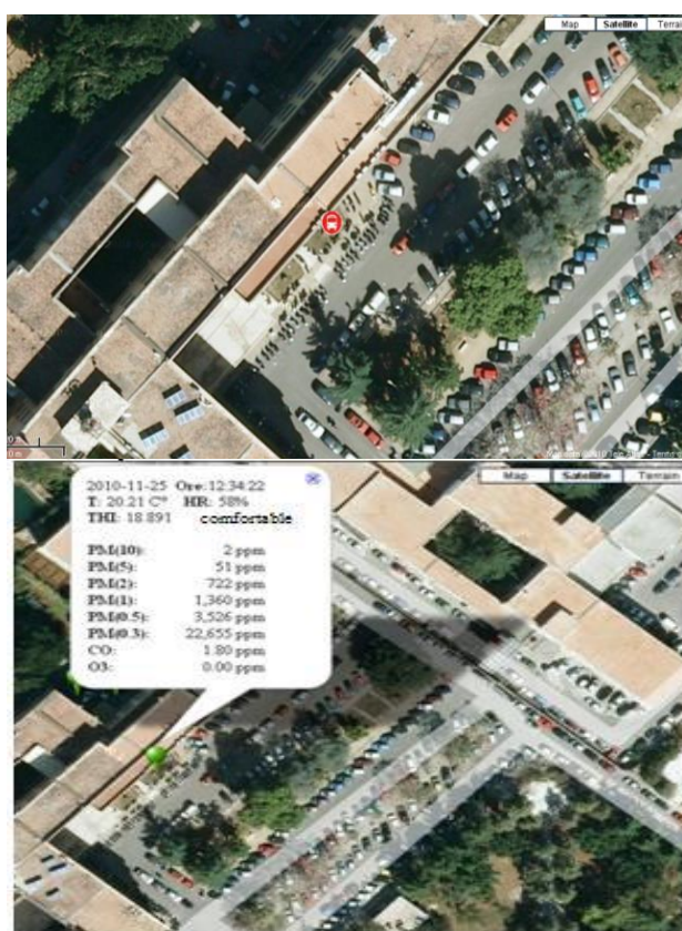
Figure 6. Real-time values detected pollutants
