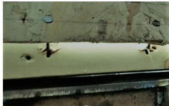
(c) Nail pulling through the panel (d) End stud lifted off the bottom plate
