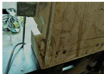
(e) Nail splitting the bottom plate (f) Bolt splitting the bottom plate
