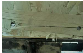
(a) Nail head embedding into the panel (b) Nail tearing out of the edges of the panel
