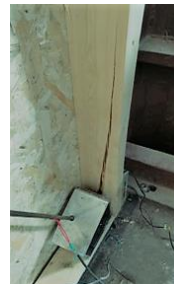
(e) Nail splitting the bottom plate (f) Bolt splitting the bottom plate
