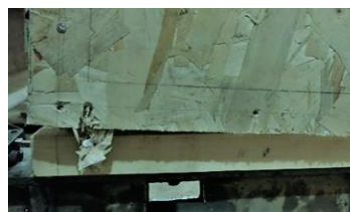
(a) Nail head embedding into the panel (b) Nail tearing out of the edges of the panel
