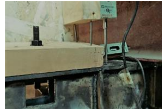
(c) Nail pulling through the panel (d) End stud lifted off the bottom plate
