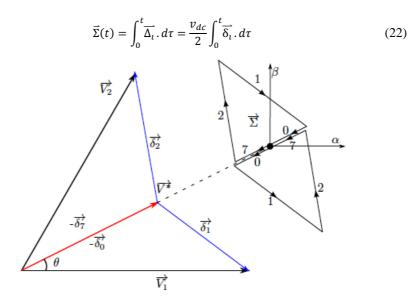
Figure 4. Example of the trajectory of the vector  $\vec{\Sigma}$  with a classical SVPWM strategy (in the sector delimited by  $\vec{V}_1$  and  $\vec{V}_2$ )
