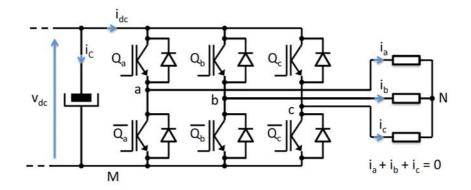
Figure 1. Battery-supplied three-phase two-level VSI
