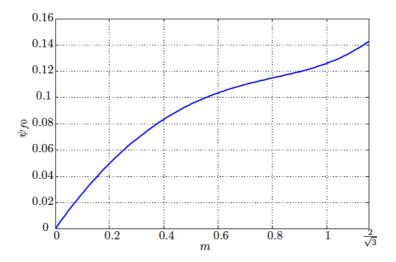
Figure 11. Harmonic flux  $\psi_f$  vs. modulation index m for the SVPWM
