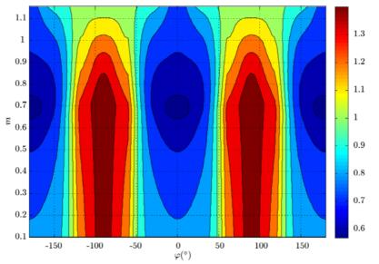
Figure 14. Cartography of the ratio between  $I_C^{RMS}$  for the Uni-DCPWM and the one obtained with the SVPWM
