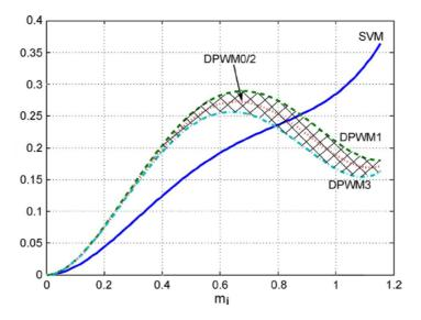
*Figure 13. Harmonic flux*  $\psi_f$  vs. *modulation index m (noted here m<sub>i</sub>)*
