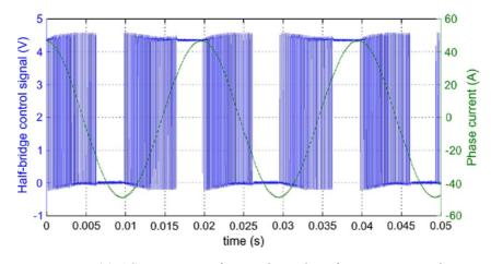
Figure 16. AC current waveform and switching function measured with the GDPWM
