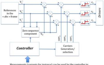
Measurements (currents for instance) can be used by the controller to modify the zero sequence component and/or the selection of carriers
