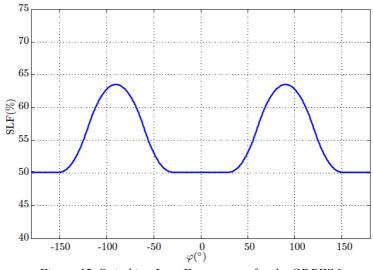
Figure 12. Switching Loss Factor vs.  $\varphi$  for the GDPWM
