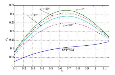
Figure 15. Harmonic flux  $\psi_f$  for the Uni-DCPWM
