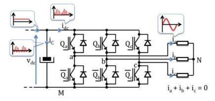
Figure 5. Separation hypothesis between AC and DC currents on the DC bus (respectively in the capacitor and the DC source)
