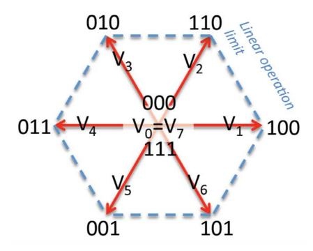
Figure 2. Constellation of instantaneous output voltage vectors in the  $\alpha\beta$  reference frame
