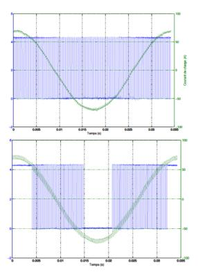
Figure 17. Comparison of AC currents for SVPWM (on the left) and Uni-DCPWM (on the right)
