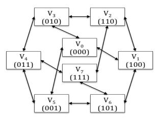
Figure 8. Useable transitions between all voltage vectors
