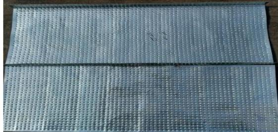
Figure 6. Typical view of absorber plates
