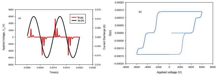
Figure 9. Simulated applied voltage and discharge current Waveforms and Lissajous figure of Filamentary DBD in He ((a) applied voltage and discharge current, (b) Lissajous figure)
