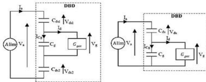
Figure 2. Classical electrical circuit of a DBD
