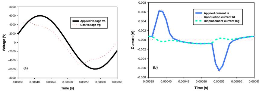
Figure 5. Wave forms a homogeneous DBD
