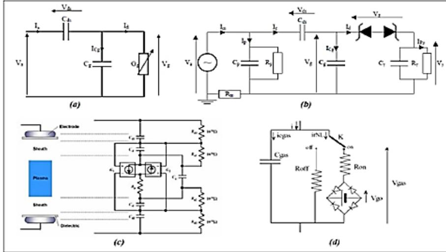
Figure 1. Example of different models of discharge circuit type: (A) Equivalent electrical diagram of the discharge (Khamphan, 2004); (B) Townsend discharge model at atmospheric pressure (Naudé, 2005); (C) Dielectric-barrier discharge (Chen, 2003); (D) Dielectric-barrier discharge (Vongphoutone et al., 2001)
