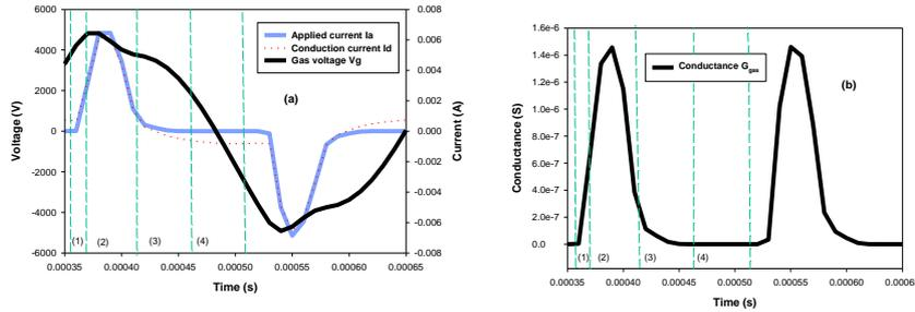
Figure 6. Typical areas of discharge: (a) Voltage/Current; (b) Conductance
