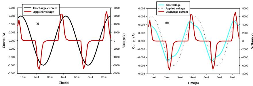
Figure 4. Time evolution of the discharge current and gas voltage during two cycles of applied field in Helium for an applied voltage of 6 kV, a frequency of 3 kHz and a gap distance of 1 mm
