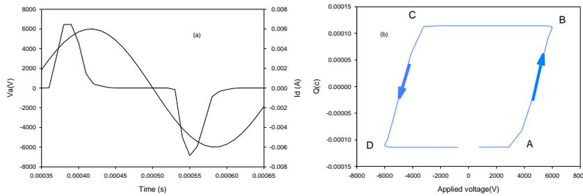
Figure 7. Simulated applied voltage and discharge current Waveforms and Lissajous Figure of Homogenous DBD in He ((a) applied voltage and discharge current, (b) Lissajous figure)
