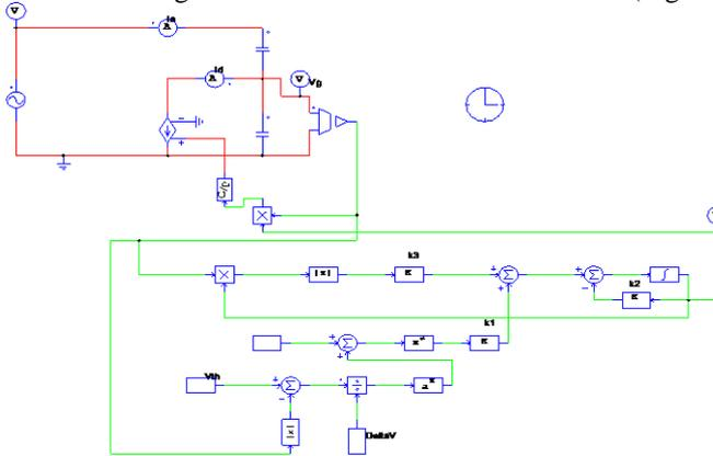
Figure 3. Electrical model of DBD in software Psim
