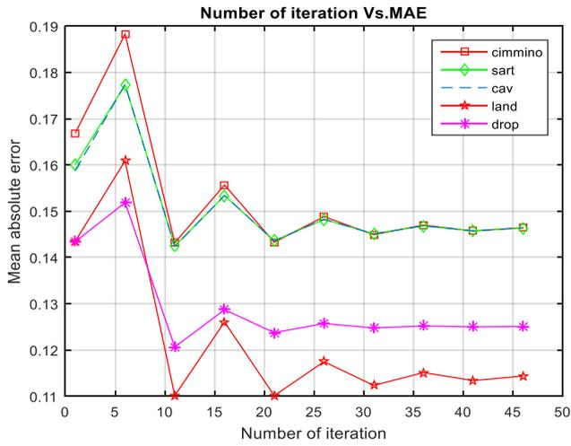
**Figure 6.** Mean absolute error between original and reconstructed image (Fan beam - test image)
