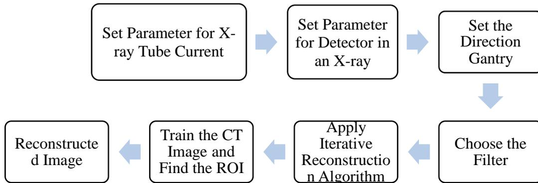
Figure 1. Block diagram of image reconstruction technique
