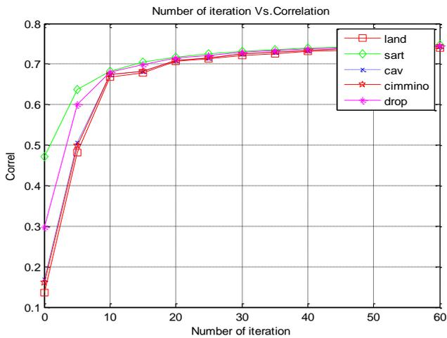
**Figure 8.** Correlation coefficient between original and reconstructed image (Fan beam - head image)
