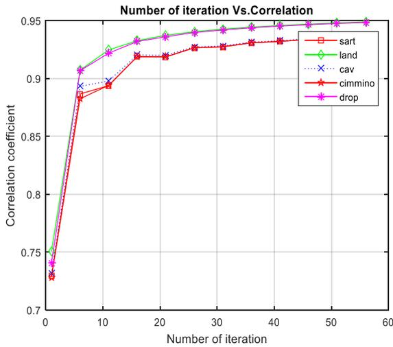
**Figure 12.** Correlation coefficient between original and reconstructed image (Parallel beam – thorax image)
