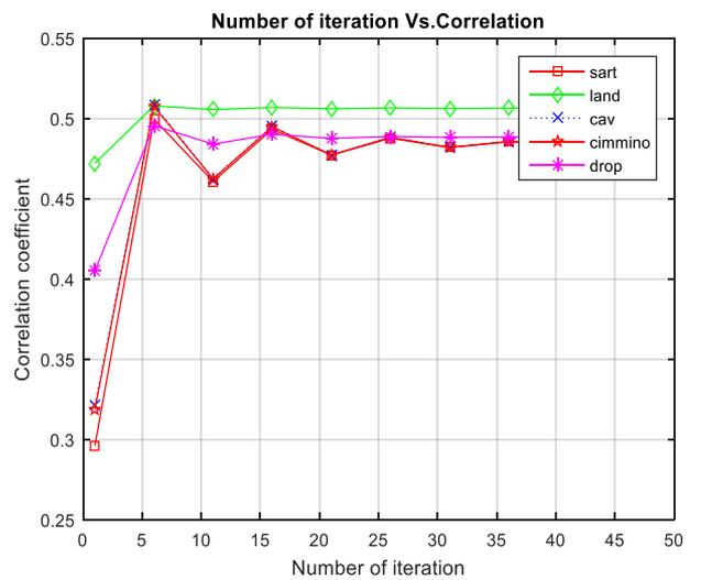
**Figure 10.** Correlation coefficient between original and reconstructed image (Fan beam - thorax image)
