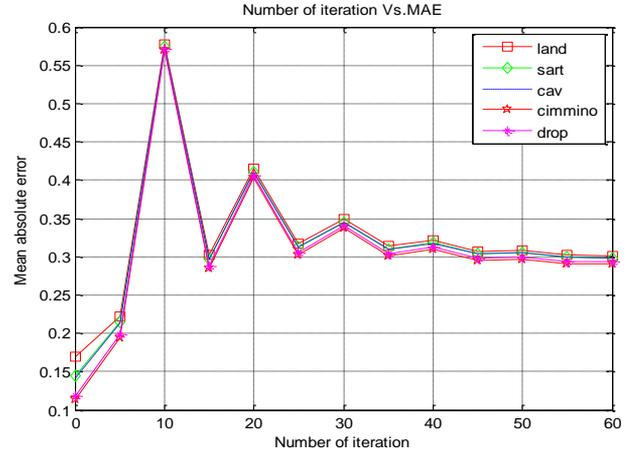
**Figure 9.** Mean absolute error between original and reconstructed image (Fan beam - head image)
