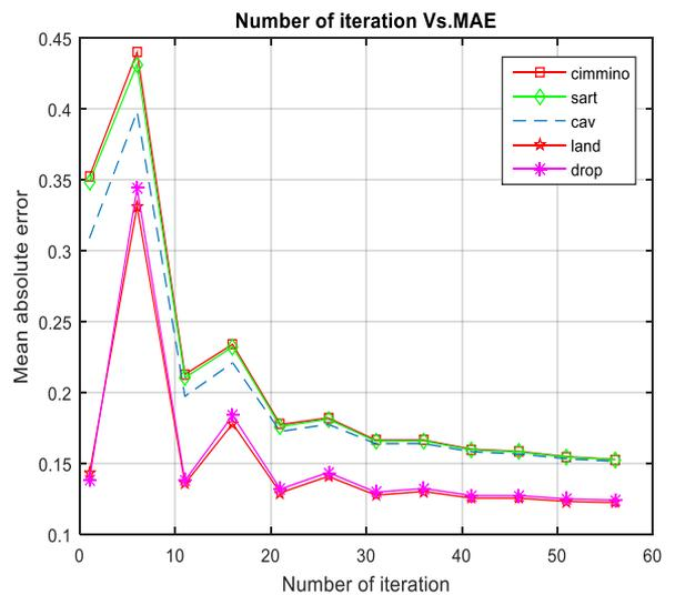
**Figure 11.** Mean absolute error between original and reconstructed image (Fan beam - thorax image)
