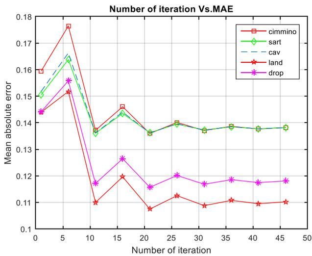
**Figure 4.** Mean absolute error between original and reconstructed image (Parallel beam - test image)
