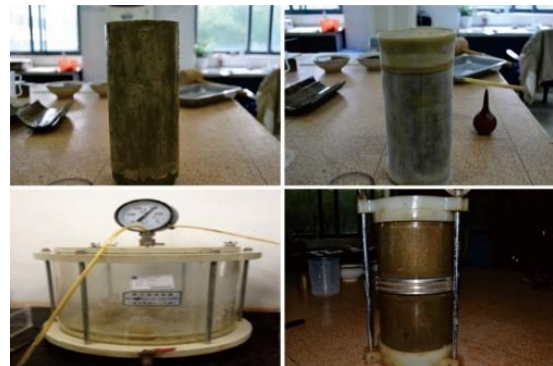
Figure 6. Preparation process of one cylindrical specimen used in the tests
