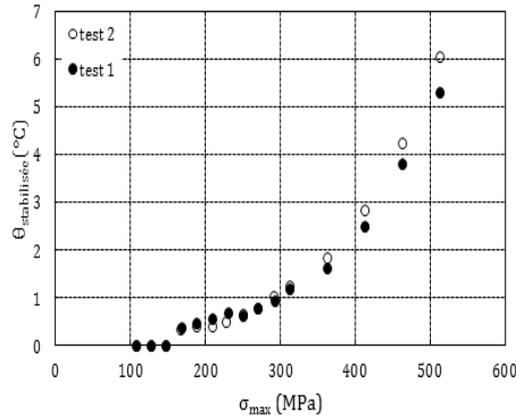
Figure 11. Self-heating curves of a  $[0]_8$  CF/PA66 woven laminated composite
