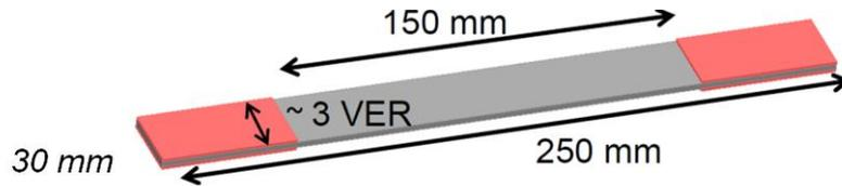
Figure 1. Specimen used for fatigue tests
