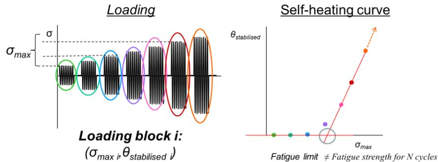
Figure 3. Explanation of fatigue limit determination: block of loading and self-heating curve
