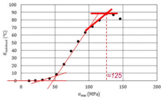
Figure 14. Determination of fatigue limits of a [45]8 CF/PA66 woven laminated composite
