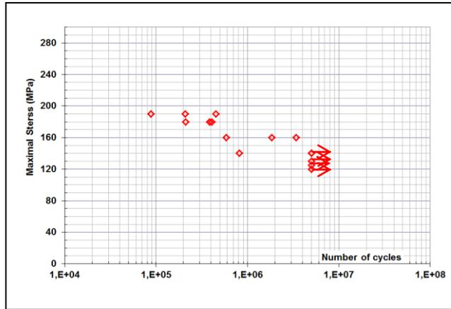
Figure 8. Experimental results for fatigue test on 45° composite
