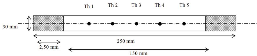
Figure 5. Specimen geometry and thermocouples location
