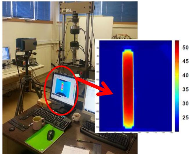
Figure 4. Temperature measurement with infrared camera
