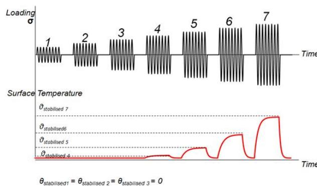
Figure 2. Description on the self-heating method
