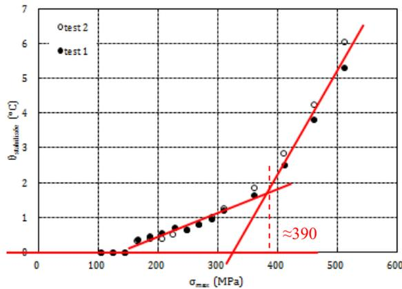
Figure 12. Determination of the fatigue limit of a PA66  $[0]_8$
