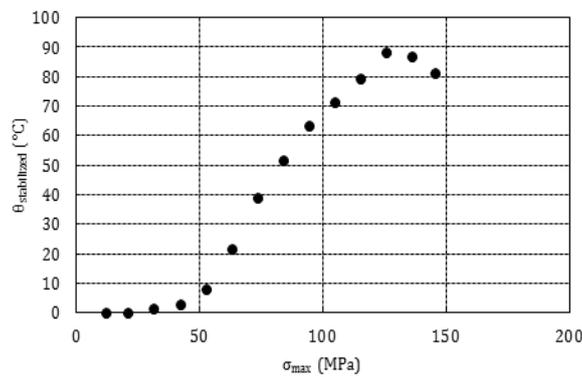
Figure 13. Self-heating curve of a [45]8 CF/PA66 woven laminated composite
