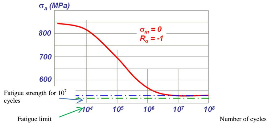
Figure 15. Difference between fatigue limit and fatigue strength
