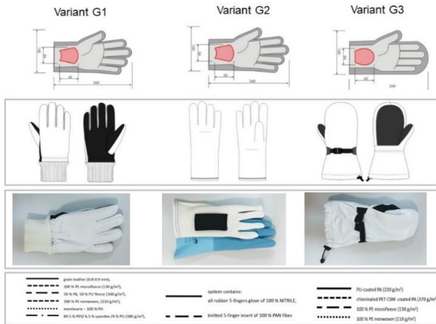
Figure 2. Design and materials used in the studied gloves
