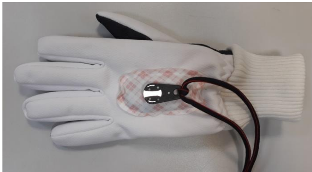
Figure 4. Location of mineral warmer and a T/RH sensor inside an inner pouch
