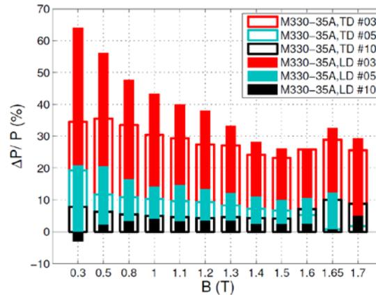
Figure 6. Loss degradation factor of the M330-35A alloy at 50 Hz
