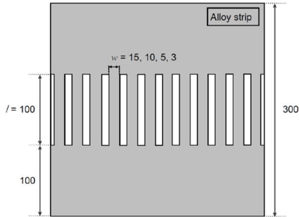
Figure 1. Punched samples preparation (the unit is millimeter)
