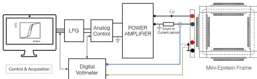
Figure 2. Scheme of the experimental setup
