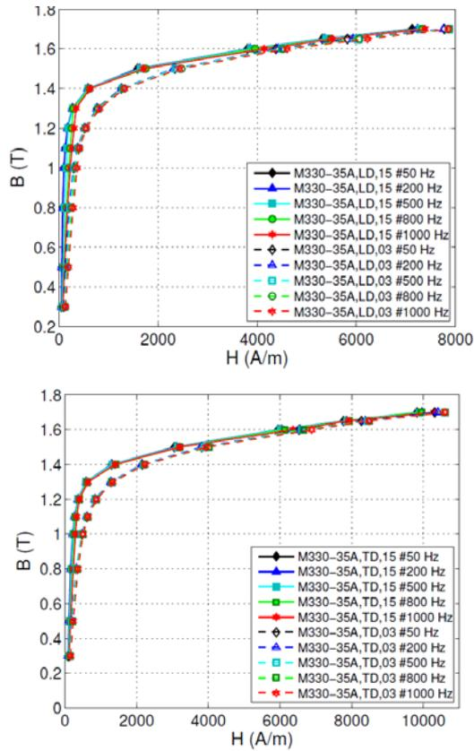
Figure 7. Frequency magnetization curves of the M330-35A alloy measured in both LD and TD directions
