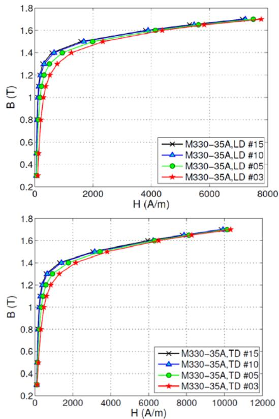
Figure 3. 50 Hz normal magnetization curves of the M330-35A alloy measured in both LD and TD directions (# w denotes the width of the sample in mm)
