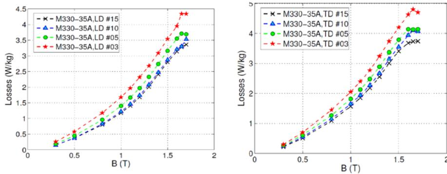
Figure 5. 50Hz loss vs induction curves of the M330-35A alloy measured in both LD and TD directions
