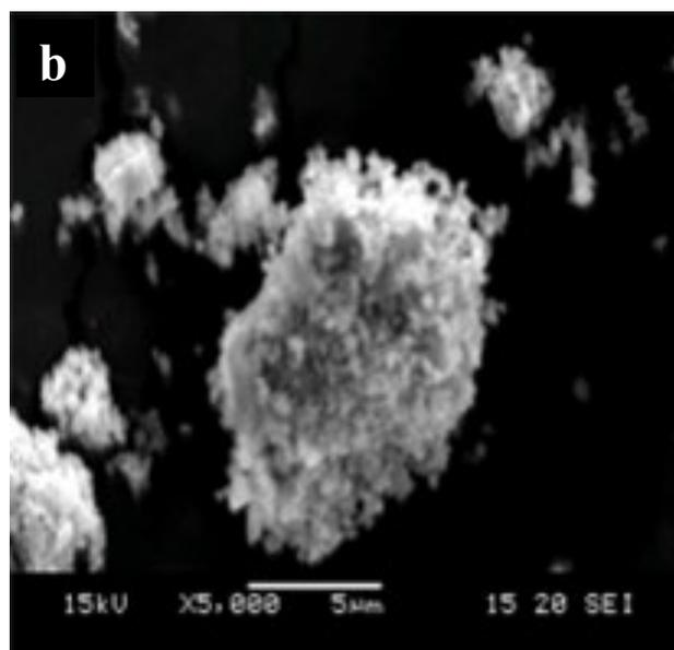
Figure 5. SEM image for  $\text{Cu}_2\text{SnS}_3$  nanoparticles prepared at 50 % of Ethylenediamine concentration.
