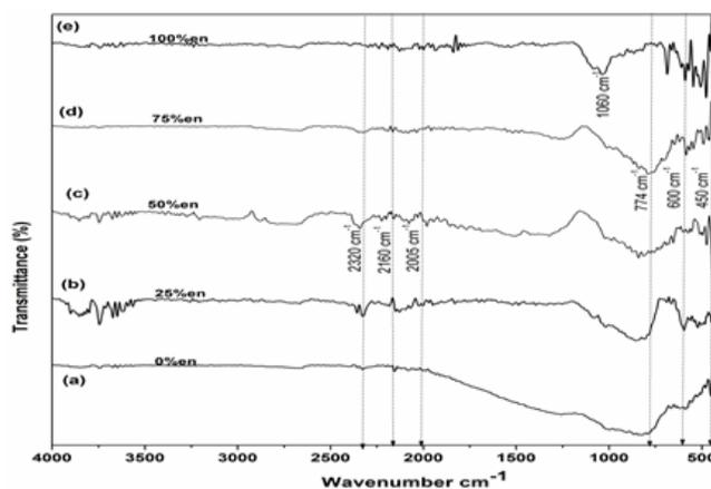
Figure 3. FTIR spectra for  $\text{Cu}_2\text{SnS}_3$  nanoparticles obtained for various ethylenediamine concentrations: (a) 0, (b) 25, (c) 50, (d) 75, (e) 100%.
