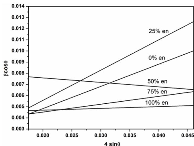
Figure 2. Williamson Hall plot for  $\text{Cu}_2\text{SnS}_3$  nanoparticles obtained for various ethylenediamine concentrations: 0 to 100 %.
