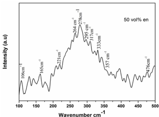
Figure 4. Raman spectra for  $\text{Cu}_2\text{SnS}_3$  nanoparticles prepared at 50 % of ethylenediamine concentration.
