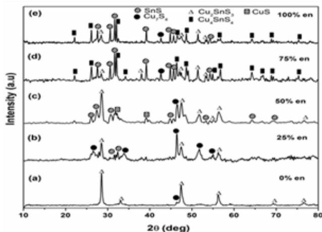
Figure 1. X-ray diffraction pattern for  $\text{Cu}_2\text{SnS}_3$  nanoparticles obtained for various ethylenediamine concentrations: (a) 0, (b) 25, (c) 50, (d) 75, (e) 100 %.
