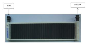
Figure 1. Integrated Planar Solid Oxide Fuel Cell (IP-SOFC).
