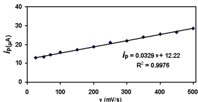
Figure 4. Plot of peak current vs scan rate
