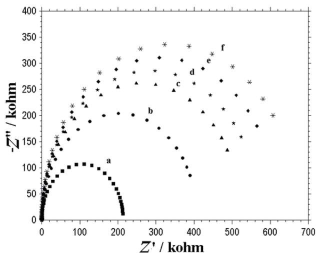
Figure 9. Impedance responses obtained at P3MT/GCE in the presence of various concentrations (a-0.2  $\mu\text{M}$ , b-3.3  $\mu\text{M}$ , c-4.29  $\mu\text{M}$ , d-5.0  $\mu\text{M}$ , e-5.5  $\mu\text{M}$ , f-6.0  $\mu\text{M}$ ) of diazepam. Amplitude: 0.005 V, frequency: 100 mHz to 100 kHz
