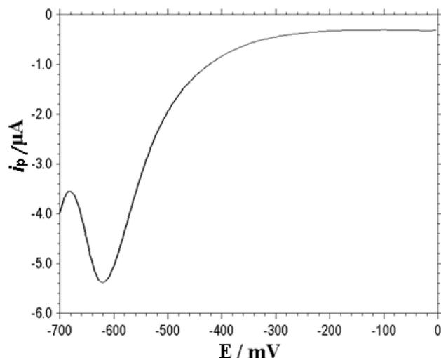
Figure 10. DPSV behaviour of diazepam under optimum experimental conditions
