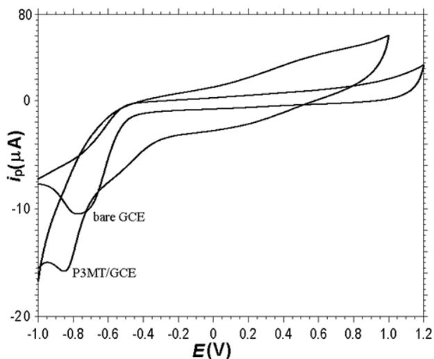
Figure 3. Cyclic voltammogram of 0.2  $\mu\text{M}$  diazepam on bare and P3MT modified GCE at pH 1.0; scan rate 0.05 V/s
