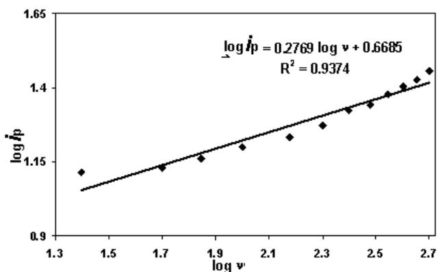
Figure 6. Plot of log peak current vs log of scan rate
