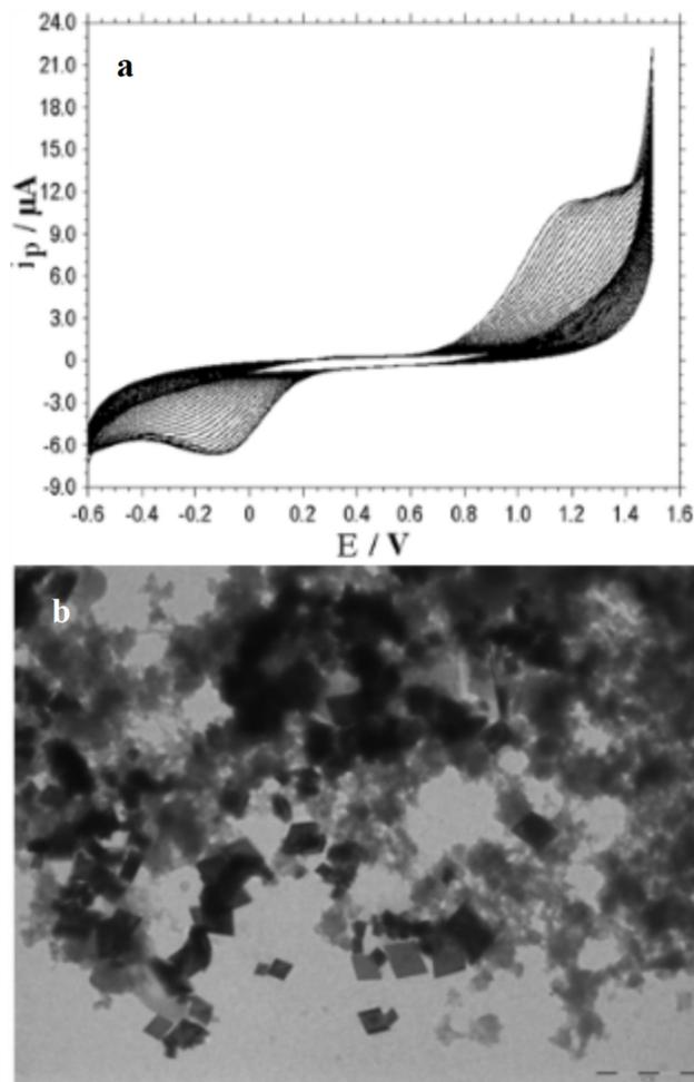
Figure 1. a. Cyclic voltammogram of 0.1M P3MT in 0.1M H<sub>2</sub>SO<sub>4</sub> at a scan rate of 0.05 V/s, b. TEM image of P3MT
