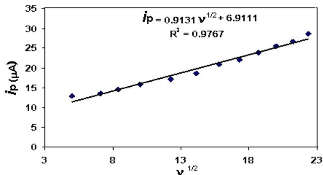
Figure 5. Plot of peak current vs log of scan rate
