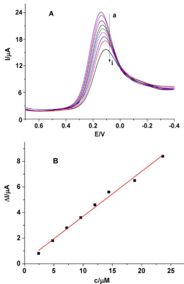
Figure 3. (A) SWVs of the MIP sensor with different concentrations of sulfamethoxazole. From a-g: 0; 2.4; 4.8; 7.2; 9.6; 12; 14.4; 18.8; 23.6  $\mu M$ . (B) Plot of the  $\Delta I_p$  versus concentration of sulfamethoxazole.
