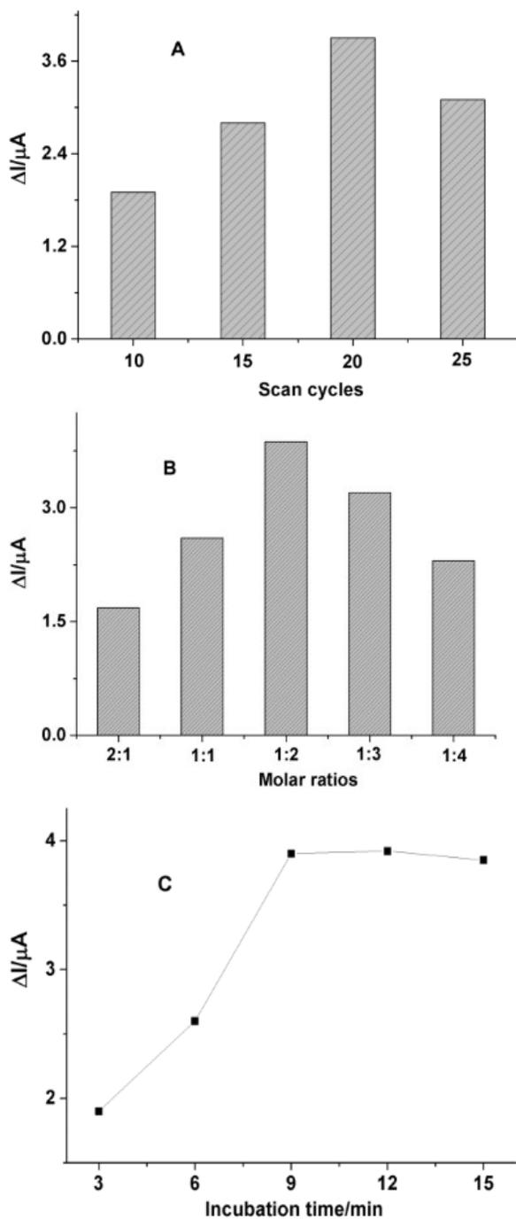
Figure 2. The effect of the scan cycles(A), the mole ratio of template molecules to functional monomers(B), and incubation time(C) on the  $\Delta I_p$  of MIP sensor.
