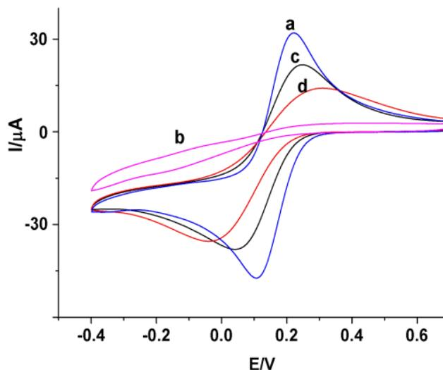
Figure 1. Cyclic voltammograms of 1.0 mM  $\text{K}_3[\text{Fe}(\text{CN})_6]$  at MWCNT/GCE (a), MIP/MWCNT/GCE without removing sulfamethoxazole (b), MIP/MWCNT/GCE after removing sulfamethoxazole (c), and MIP/MWCNT/GCE after incubation with sulfamethoxazole (d).
