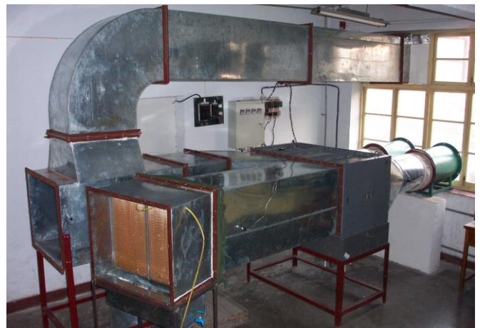
Figure 2 Evaporative cooling air conditioning system schematic diagram
