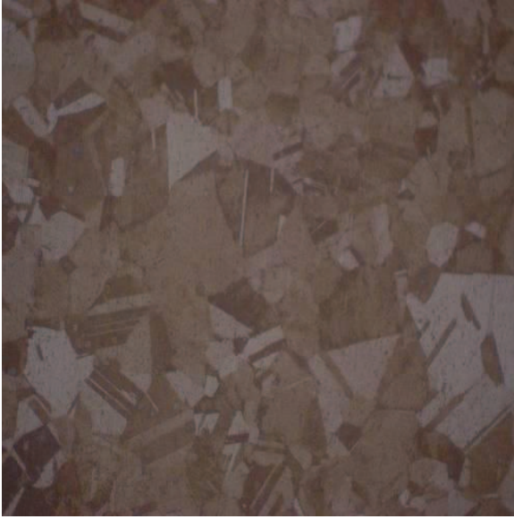
FIG.2. OPTICAL MICROGRAPH OF FAILED BLADE MATERIAL (200X)
