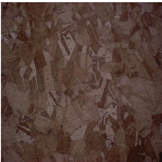
FIG.1. OPTICAL MICROGRAPH OF VIRGIN BLADE MATERIAL (200X)
