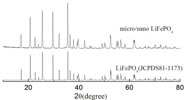
Figure 1. XRD patterns of micro/nano  $\text{LiFePO}_4/\text{C}$  composite material
