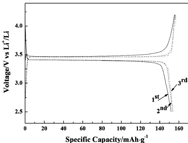
Figure 3. charge/discharge voltage profiles at 0.1 C for the first 3 cycles
