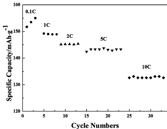
Figure 4. Rate performance of micro/nano LiFePO<sub>4</sub>/C
