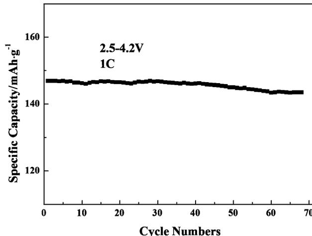
Figure 5. Cycle performance of micro/nano LiFePO<sub>4</sub>/C at 1 C in the voltage range of 2.5-4.3 V (vs. Li/Li<sup>+</sup>)
