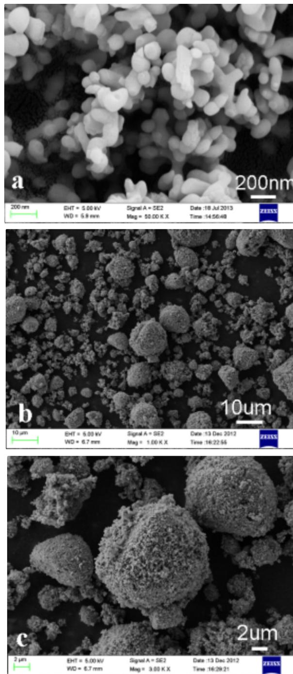
Figure 2. SEM images of nano  $\text{FePO}_4$  (a) and micro/nano (b and c)  $\text{LiFePO}_4/\text{C}$  composite material
