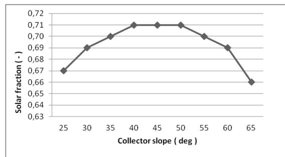
**Figure 11.** Solar fraction at different collector slope
