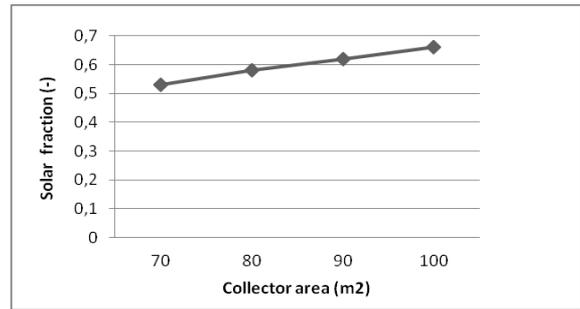
**Figure 13.** Solar fraction at different collector's surface
