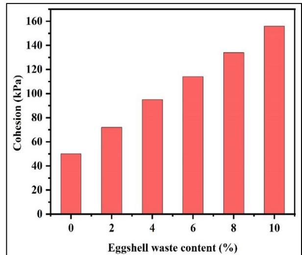
Figure 9. Effect of eggshell powder on cohesion
