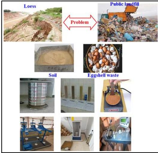
Figure 4. Schematic diagram of experimental program
