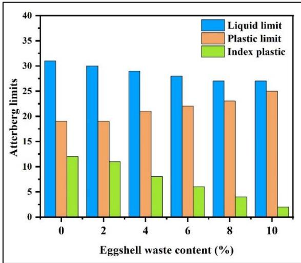
Figure 7. Effect of eggshell powder on Atterberg’s limit of soil
