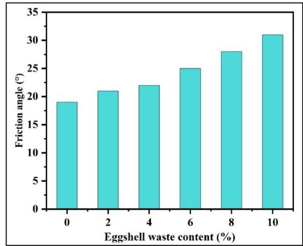
Figure 8. Effect of eggshell powder on friction angle
