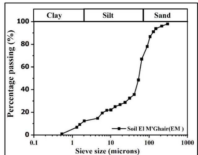
Figure 2. Grain-size distribution curves of loess soil
