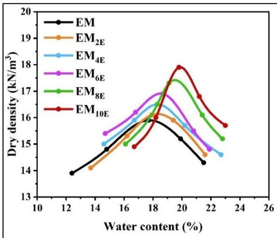
Figure 5. Effect of eggshell powder on Proctor parameters of soil
