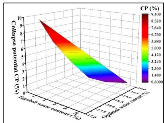
Figure 6. Effect of eggshell powder on collapse potential of soil
