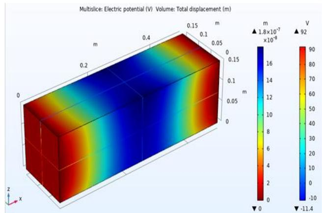
Figure 6. Electric potential and total displacement in state 3
