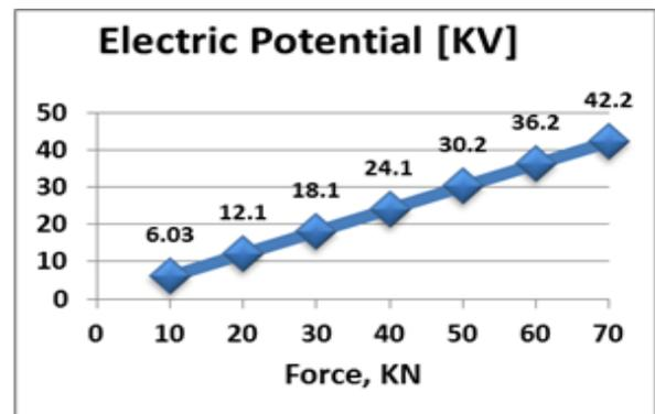
Figure 10. Electric potential result of PVDF
