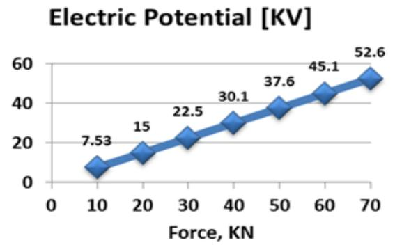
Figure 8. Electric potential result of PZT-2
