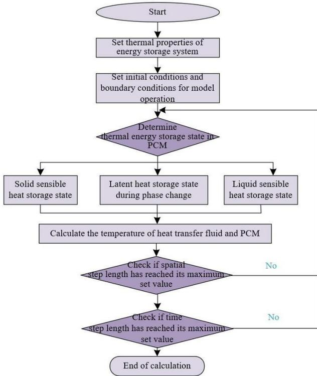
**Figure 2.** Numerical calculation flowchart for energy storage module in DESS
