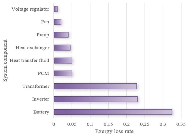
**Figure 7.** Exergy loss rates of different components in DESS for power distribution networks
