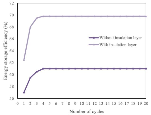
**Figure 4.** Variation in energy storage efficiency of DESS with and without insulation layers across multiple operational cycles
