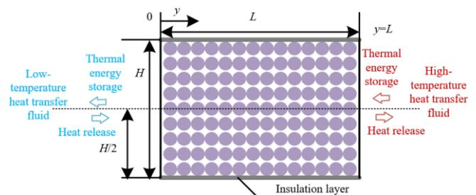
**Figure 1.** Schematic diagram of numerical computation for energy storage module in DESS
