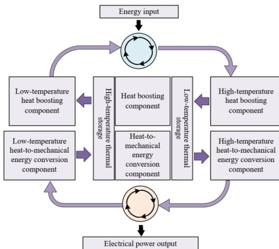
Figure 3. Energy transfer process in DESS
