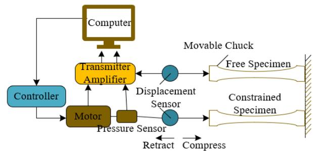
Figure 4. Temperature-stress testing system for prefabricated box culvert specimens
