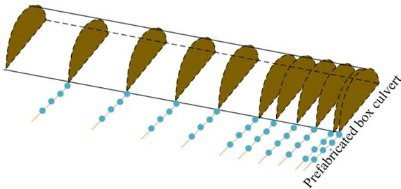
**Figure 1.** The longitudinal sensor placement in prefabricated box culverts
