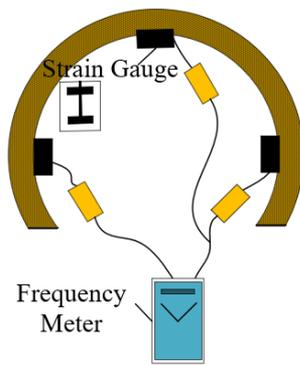
**Figure 3.** Stress and strain monitoring point layout diagram
