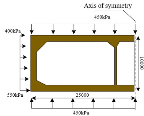
**Figure 2.** Side cross-sectional load condition of prefabricated box culvert specimens
