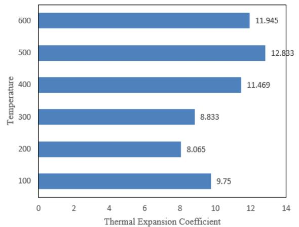
**Figure 6.** Thermal expansion coefficients of prefabricated box culvert specimens under three-dimensional stress state
