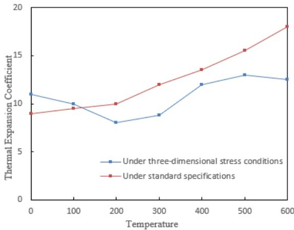
**Figure 7.** Comparison of thermal expansion coefficients of prefabricated box culvert specimens under different states
