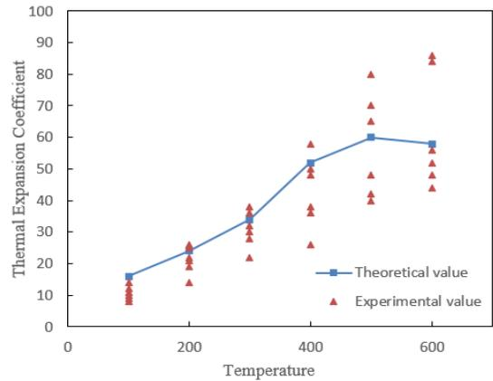
**Figure 9.** Comparison of theoretical and experimental values of thermal expansion stress of prefabricated box culvert specimens under three-dimensional stress state
